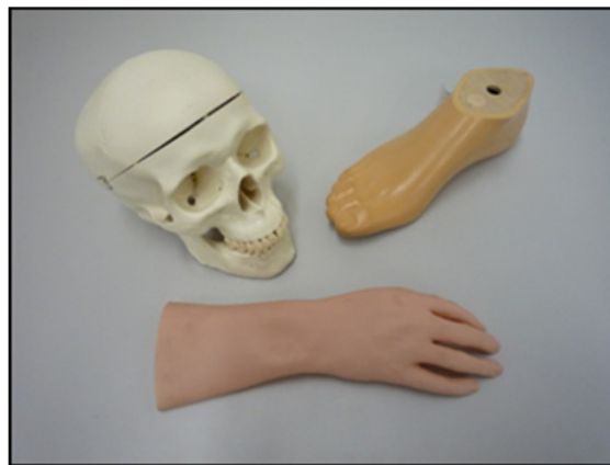
Figure 8. Samples from the field of biomedical engineering evaluated by metrotomography (epithesis and plastic human skull).
