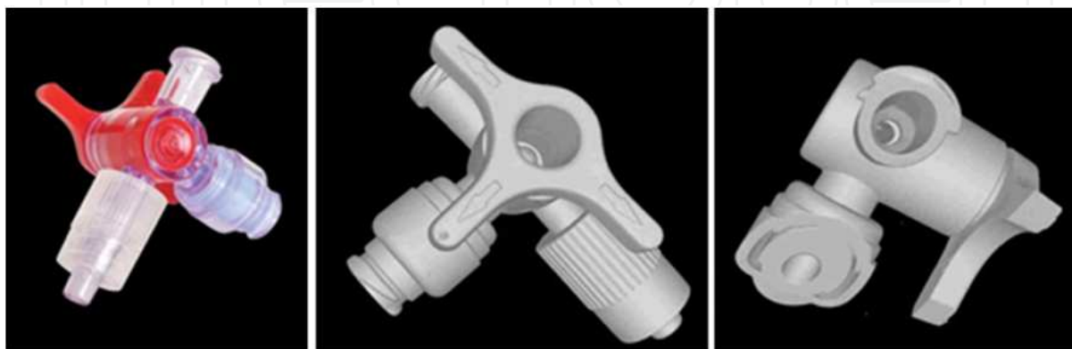
Figure 4. CAD models of the multidirectional valve – presentation of the reverse engineering.
