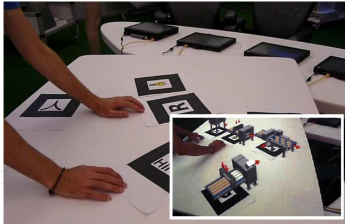
Figure 15. The Augmented Reality Table. The picture shows the markers and (inset) the virtual models projected on top of these markers.
