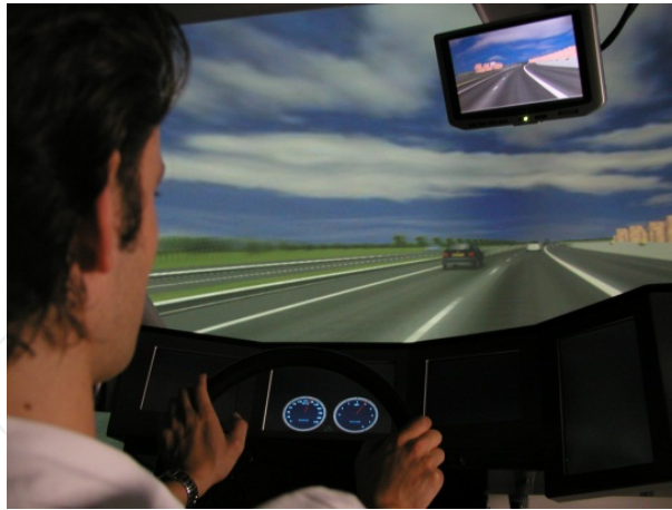
Figure 2. The driving simulator used for testing lane-change support systems, also showing the configurable dashboard.
