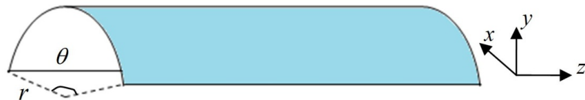
Figure 7. A curved armchair graphene nanoribbon with the tubular shape. \theta is the central angle and r is the curved radius of the nanoribbon.
