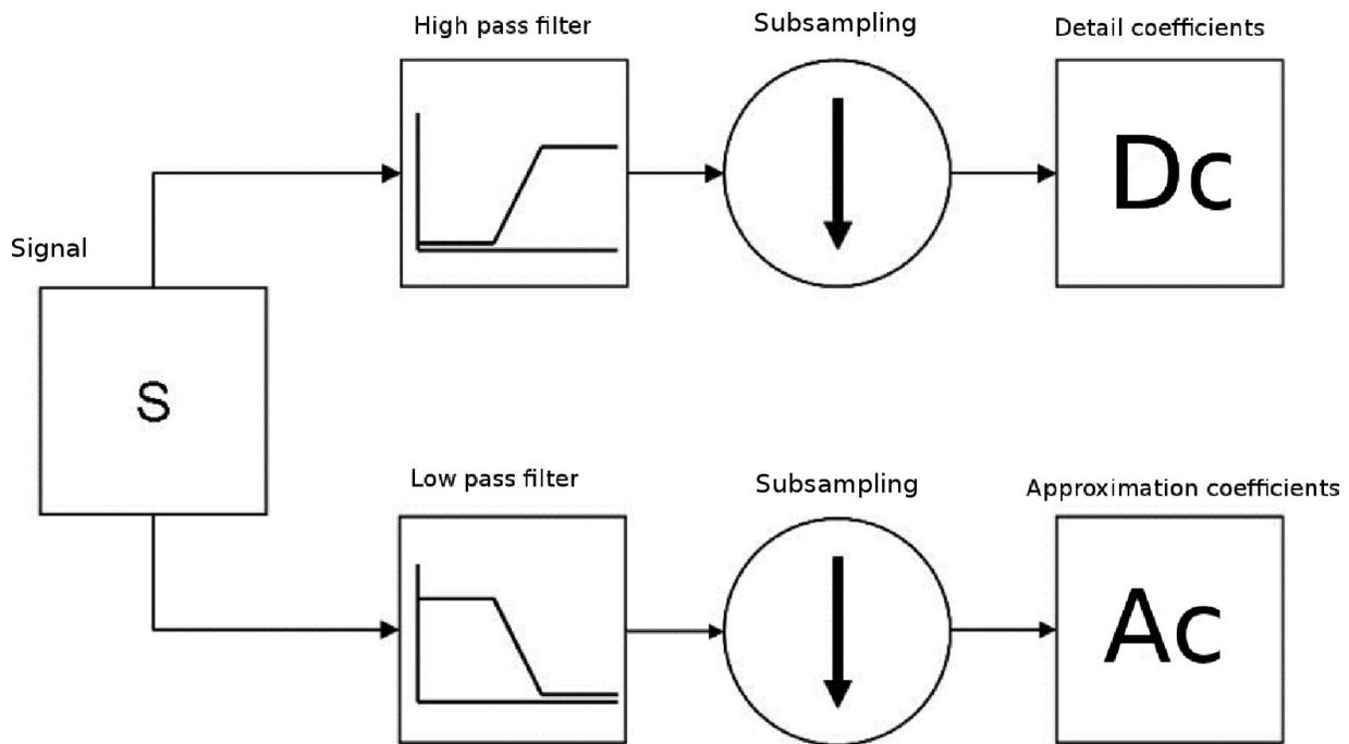
**Figure 9.** Algorithm for the Discrete Wavelet Transform
