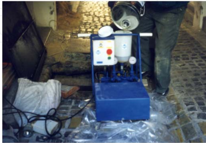
Figure 1. Two component electric grouting pump DV 97.
