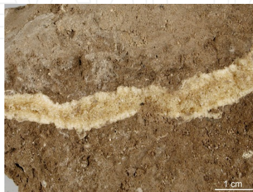
Figure 7. Claquage texture – fine-grained soil fractured hydraulically with claquage fissure, which is filled with PUR-binder.
