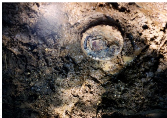
Figure 22. Borehole with contaminated water seepages
