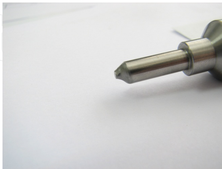
Figure 10. Mixing head needle corrosion by EG
