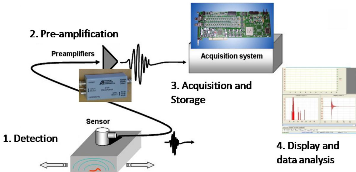
**Figure 3.** Schematic diagram of the AE test system
