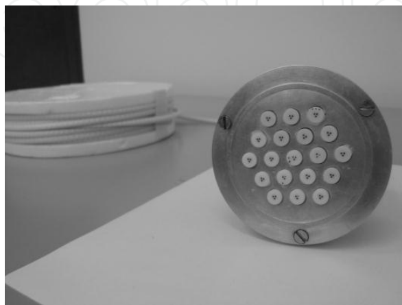
Figure 10. Inserts with optical fibres to be used in a fibres collector plate. Each insert can have several fibres.
