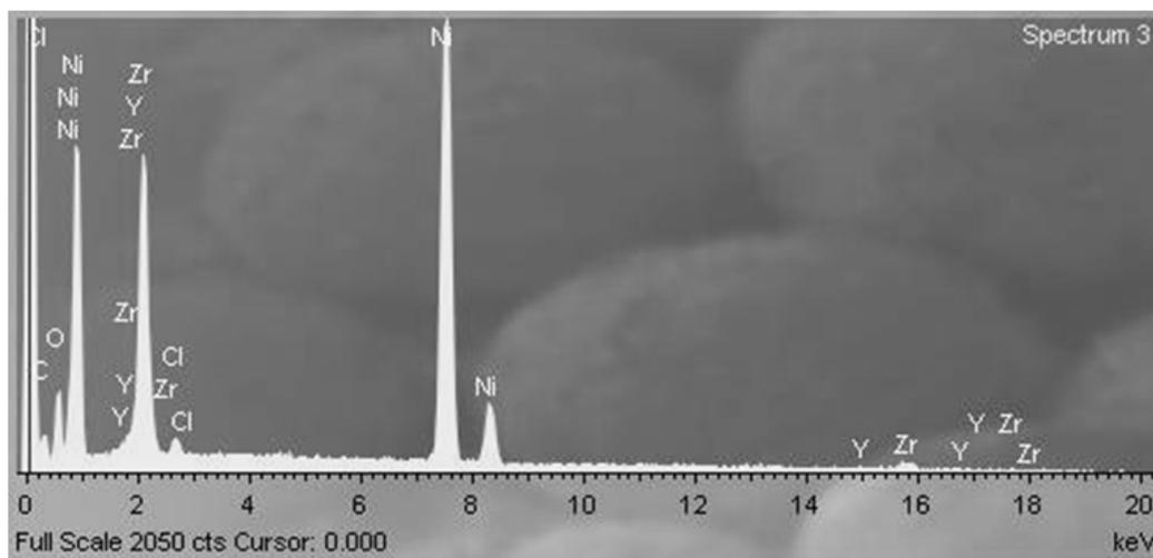
**Figure 5.** EDX spectrum showing presence of the corresponding EN co-deposition
