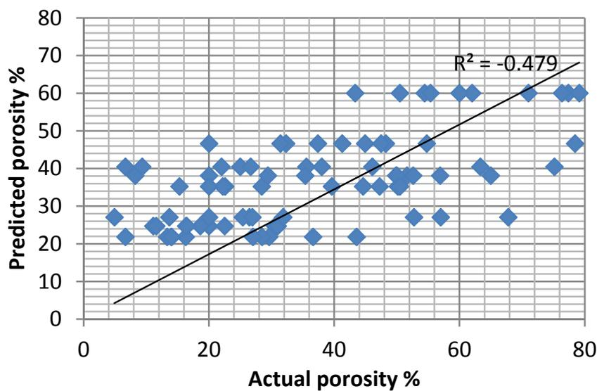
**Figure 14.** Comparison of experimental and predicted values for porosity content
