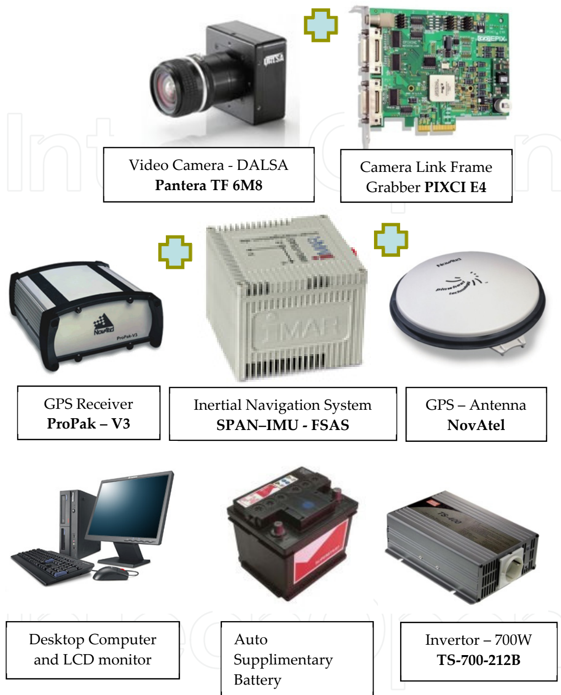
Figure 13. The components of the Mobile Slide Monitor
