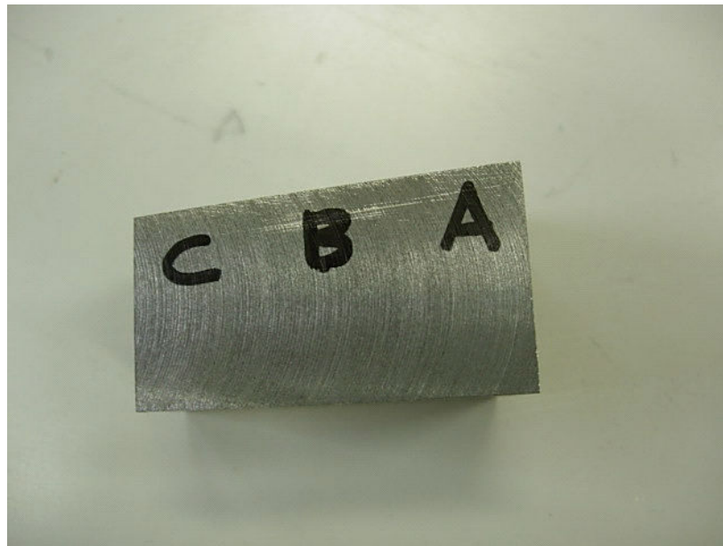
Figure 14. Three measuring points of a specimen (A: largest, B: middle, C: smallest in thickness).
