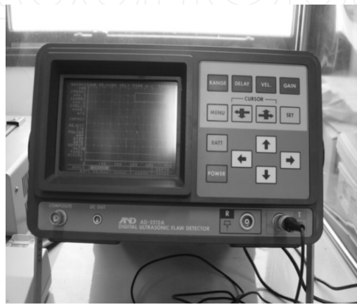
Figure 4. Ultrasonic velocity tester used.
