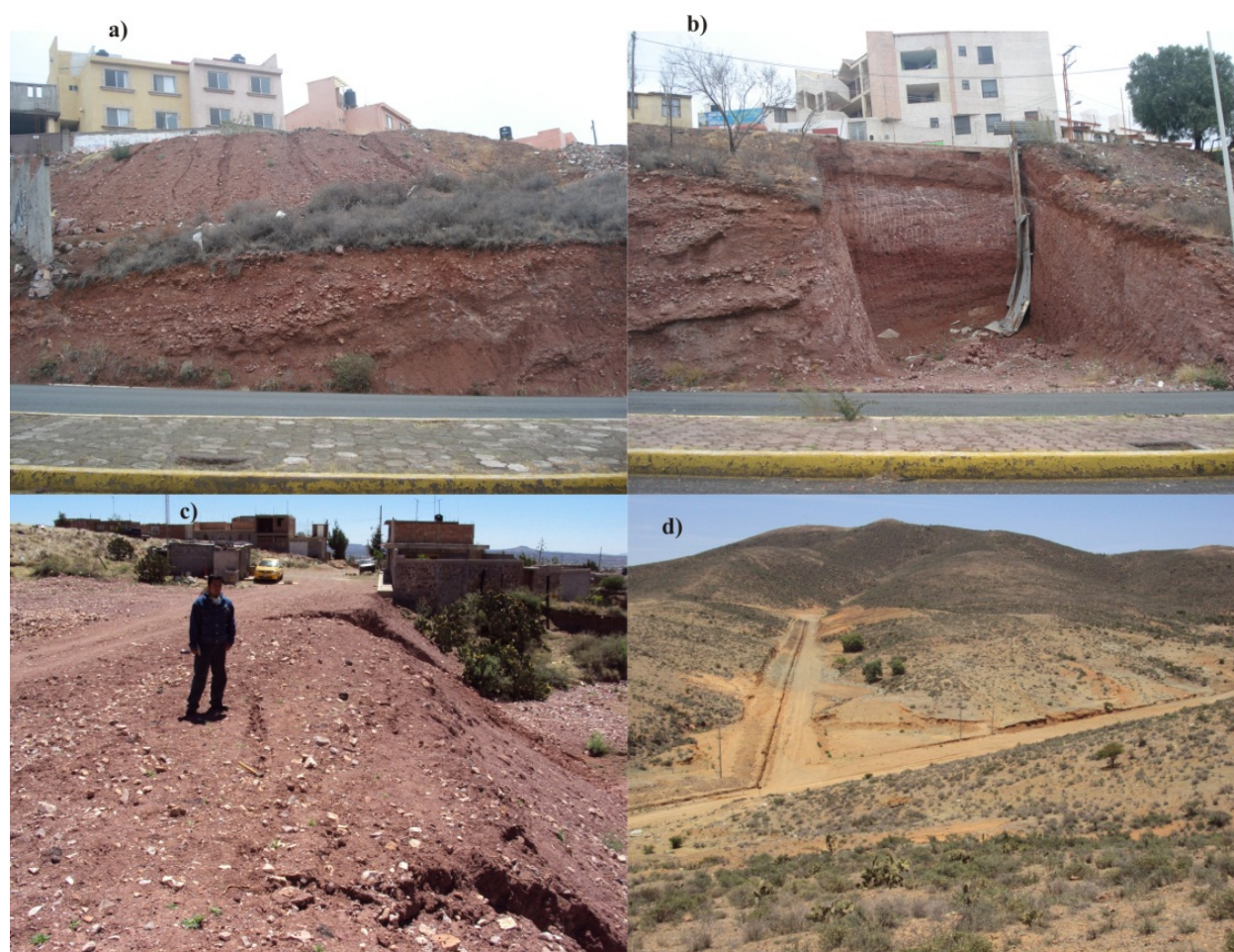
Figure 13. Field verification of the proposed model for hazardous zones associated with erosion. a) Moderate erosion zone; in the filling deposit can be seen gullies formed after the rainy season; whereas the conglomerate is affected by differential erosion. b) Intense erosion zone. An excavation was made
