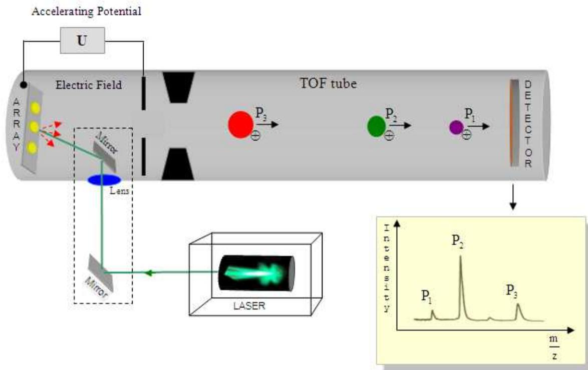
**Figure 11.** Surface enhanced laser desorption ionisation– time of flight (SELDI-TOF). The proteins are “eluted” from the matrix array by laser desorption and ionization. The ionized proteins are accelerated in the electric field and enter the TOF tube, according to their mass to charge ratio, with different velocities and each detection signal is represented by a peak in the mass spectrum.
