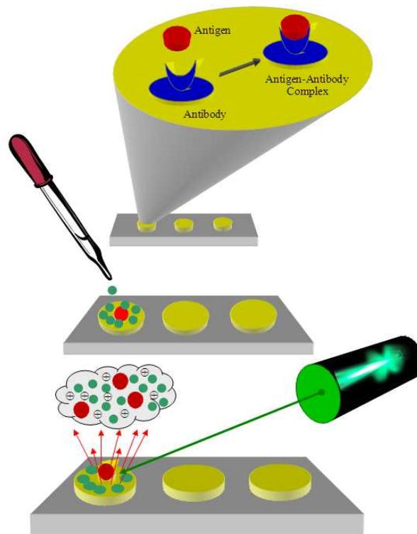
**Figure 12.** The chip array (aluminium carrier) contains immobilized GAD 65 antibodies, enabling it to focus specially on the GAD 65 antigen. The sample molecules are mixed with small matrix molecules, facilitating desorption and ionization of the proteins in the mixture. The laser pulse excites the matrix molecules; the serum molecules are liberated from the array and protonized.
