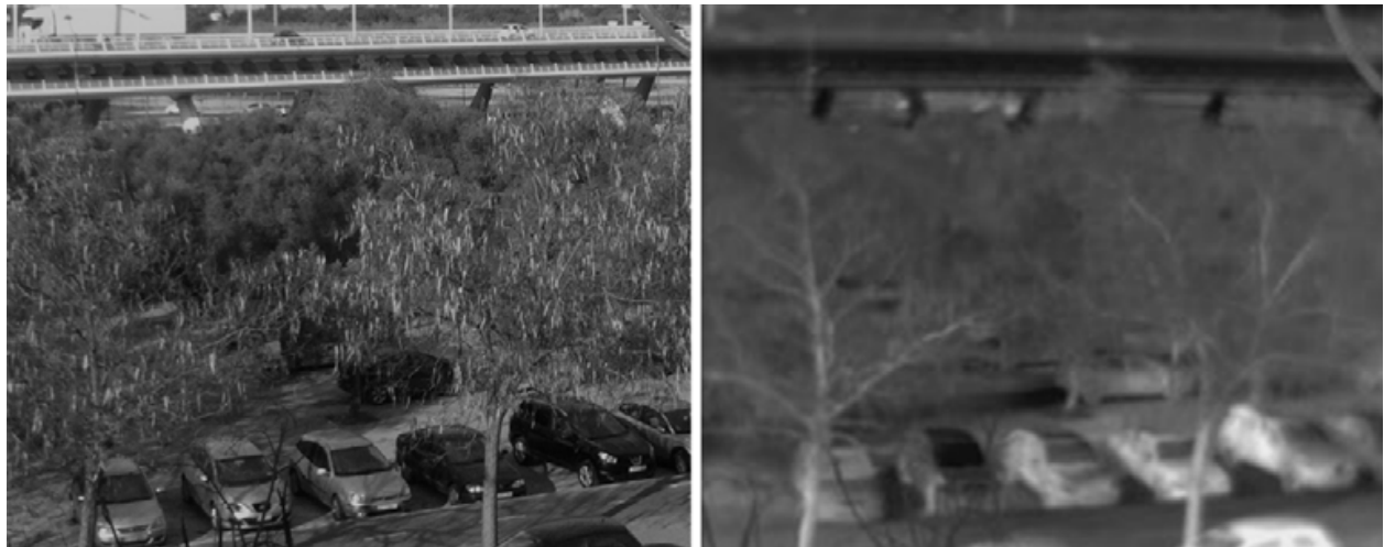
Fig. 2. Two images of the same scene but taken with different cameras one visual camera (left) and one FLIR ThermoCam P20 infrared camera (right)
