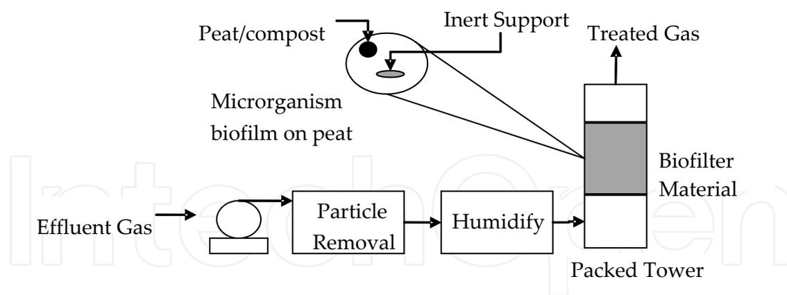
**Figure 4.** Illustrative depiction of a typical biofilter operation.
