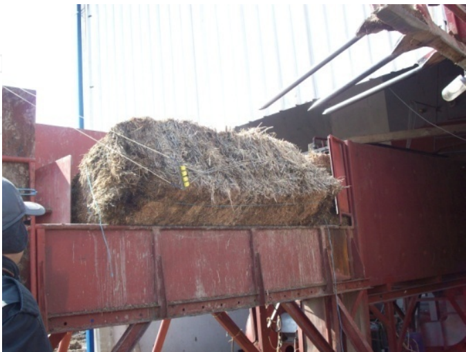
Figure 22. Thermocouples on the bale in feeding system
