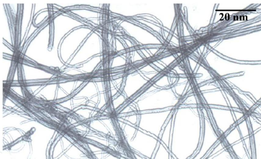
**Figure 12.** TEM image of the as-grown MWCN synthesized in LiCl [58].
