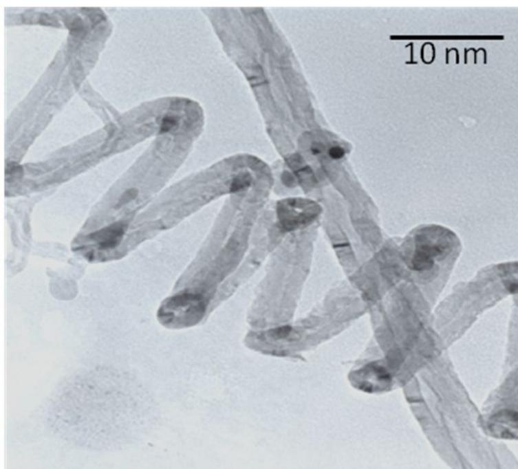
**Figure 4.** Carbon nanotubes produced in LiCl 0.25 N [51].
