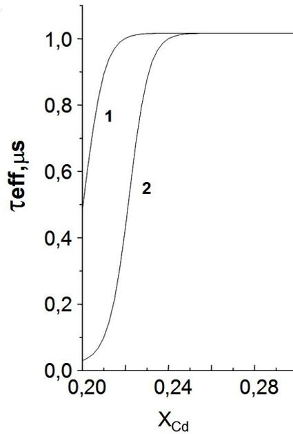
**Figure 16.** The effective lifetime  $\tau_{eff}$  in MCT HES. The dislocation density-  $5 \cdot 10^7 \text{ cm}^{-2}$ ,  $C_d = 60 \text{ s/cm}^2$ . The surface recombination velocity: 1 -  $10^3 \text{ cm/s}$ , 2 -  $10^5 \text{ cm/s}$ .
