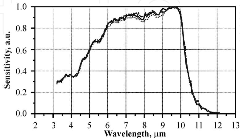
Figure 34. Spectral responsivity 320 $\times$ 240 PV FPA.
