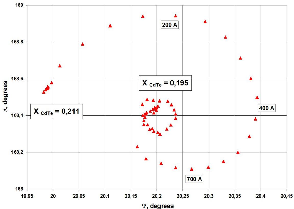
**Figure 12.** The evolution of ellipsometric parameters  $\Psi$  and  $\Delta$  in  $\Psi$ - $\Delta$  plane at initial stage of growth: triangular – experimental data; dotted line – calculated data. The цифры – MCT thickness.
