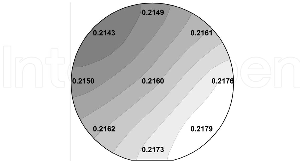
**Figure 11.** The MCT composition uniformity over the surface area of 3" in diameter GaAs substrate measured by transmission spectra. The mean value  $\langle X_{\text{CdTe}} \rangle = 0.2164$  and standard deviation  $\delta \langle X_{\text{CdTe}} \rangle = 0,0036$ .
