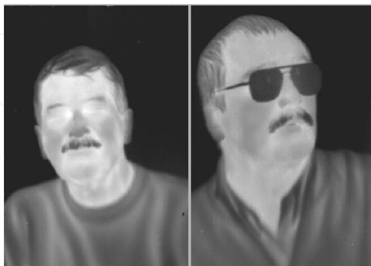
Figure 36. Thermal images 320×240 PV FPA.
