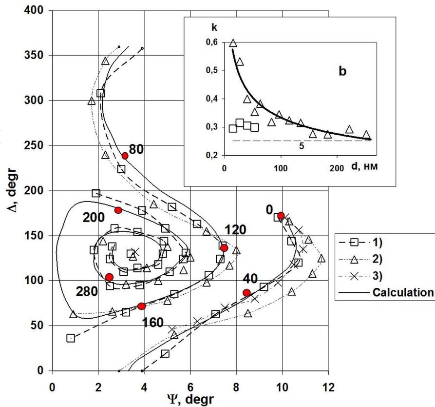
**Figure 8.** The variation of ellipsometric parameters  $\Psi$  и  $\Delta$  at CdTe growth (001)GaAs for 3 samples: squares, triangular and crosses– experimental data; solid lines – calculation data. Figures near curves – CdTe layer thickness. In insert – the dependence of adsorption factor on thickness for case of essential differences (triangular) and good agreement (squares) between experiment and calculation respectively.
