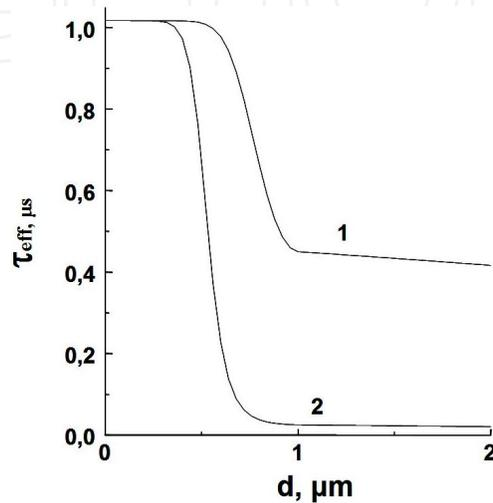
**Figure 17.** The changing of effective lifetime  $\tau_{eff}$  on etching graded wide gap layer thickness  $d$  for MCT HES:  $x_{Cd}^s = 0.3$ ,  $n_d = 5 \cdot 10^7$  cm<sup>-2</sup>. The surface recombination velocity: 1 -  $10^3$  cm/s, 2 -  $10^5$  cm/s.
