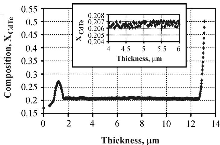
**Figure 15.** MCT composition profile throughout the thickness with narrowgap+widegap layer at the interface and widegap at the surface measured by AE *in situ*. In insert – variation of MCT composition in MCT volume.
