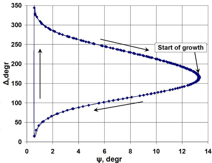
**Figure 5.** The changing of ellipsometric parameters  $\Psi$  and  $\Delta$  at growth of high quality ZnTe layer at optimal growth conditions. The points – experimental data. The rows show the direction of changing  $\Psi$  and  $\Delta$  at increasing ZnTe thickness.
