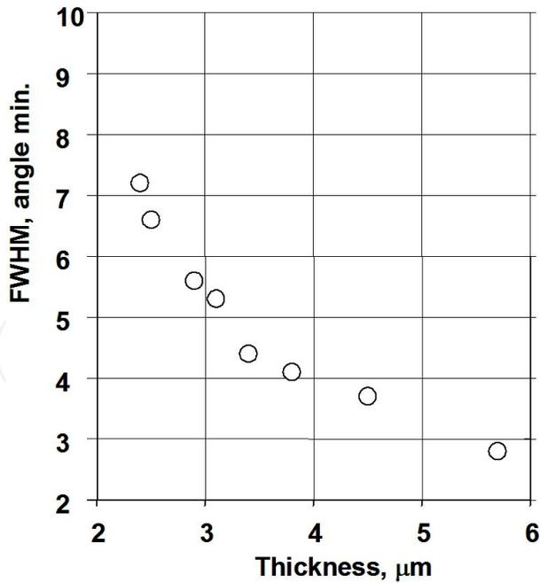
Figure 10. The dependence of FWHM on CdTe thickness.
