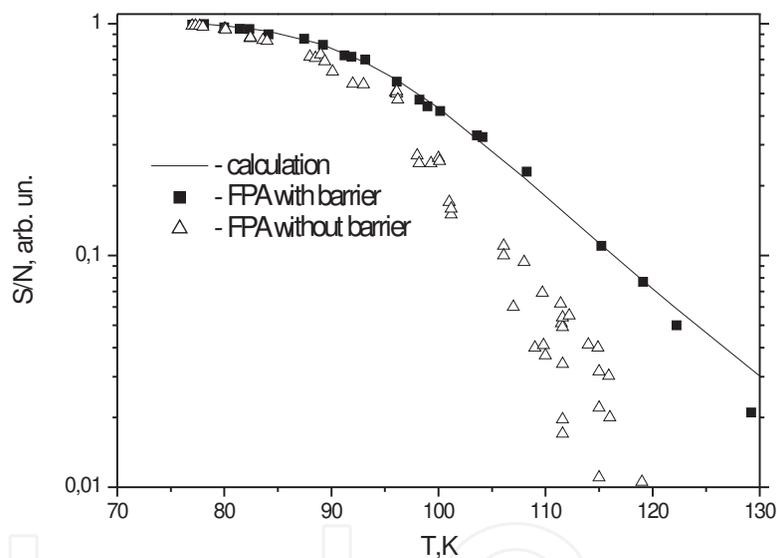
**Figure 40.** The ratio of  $S/N$  on temperature. Squares – FPA on p-p MCT HES. Triangles – FPA on p-type MCT HES. Solid curve – calculation.
