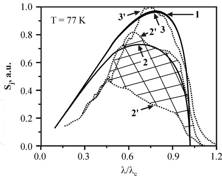
**Figure 20.** The calculated (solid 1,2,3) and experimental (dashed 1',2', 3') A-W of diodes sensitivity ( $S_j$ ) normalized to  $\lambda_c$ . Numerals are mean number MCT type on fig.19. Crosshatched region is deviation for type 2.
