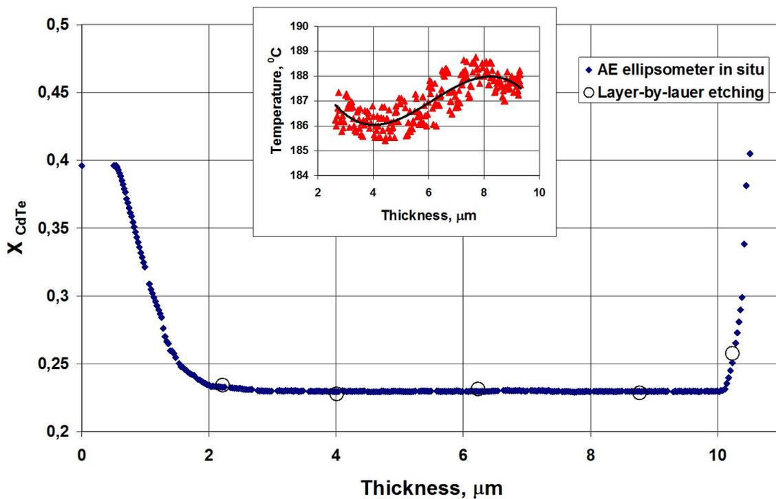
**Figure 13.** The distribution of MCT composition throughout the thickness measured by AE *in situ*. Open circles – MCT composition measured by transmission spectra at layer-by-layer chemical etching. In insert – variation of growth temperature during MCT growth.
