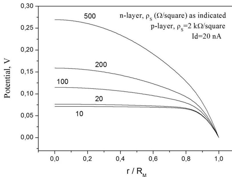
**Figure 23.** The numerical calculation data of potential distribution in 640×512 PV FPA p-type on dependence of resistance of high conductivity layer. The photocurrent of diodes is 20 nA.
