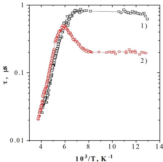
**Figure 18.** The temperature dependences of lifetime for n-type MCT HES with MCT composition in absorber layer 0,215 mole fraction CdTe: 1) – with graded wide gap layers; 2) – after chemical moving of upper graded wide gap layer.
