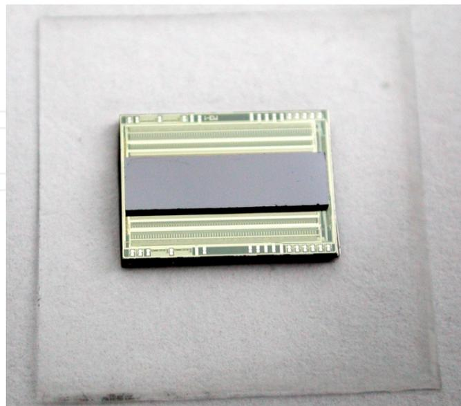
**Figure 30.** The photo view 288x4 PV FPA hybrid assembly.
