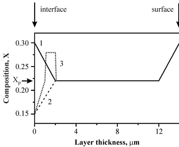
**Figure 19.** MCT composition ( $X$ ) distribution throughout the thickness with graded widegap layer at the surface and different layer at the interface: type 1 – widegap (solid line); type 2 – narrowgap (dotted line); type 3 – narrow gap + widegap (pointed line).
