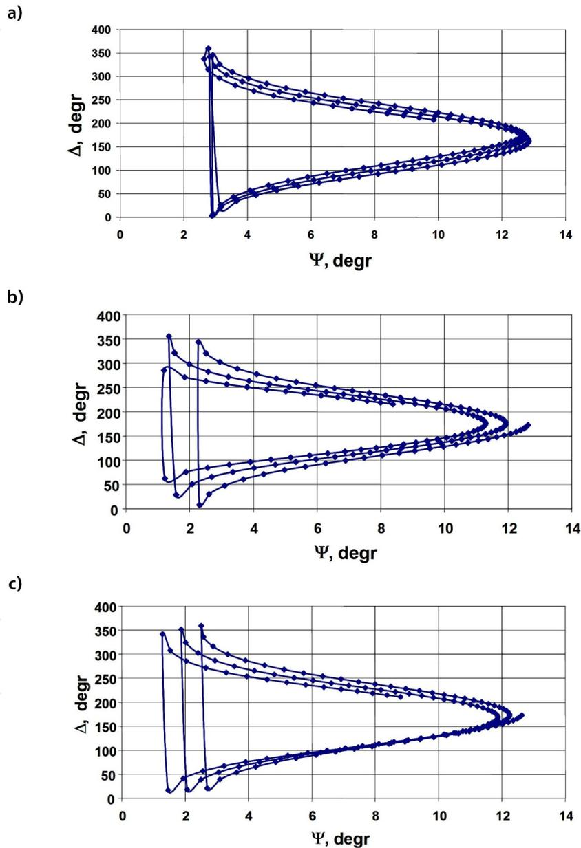
**Figure 6.** The calculation data of changing of ellipsometric parameters  $\Psi$  и  $\Delta$  at ZnTe growth on GaAs: a – roughness changes from 0 nm up to 5 nm A; b – absorption factor  $k=0.05$ ; c – roughness changes from 0 nm up to 2,5 nm, absorption factor  $k=0.03$ .
