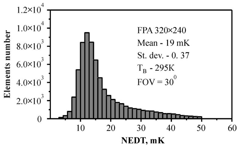
Figure 35. NEDT histogram of 320×240 PV FPA.
