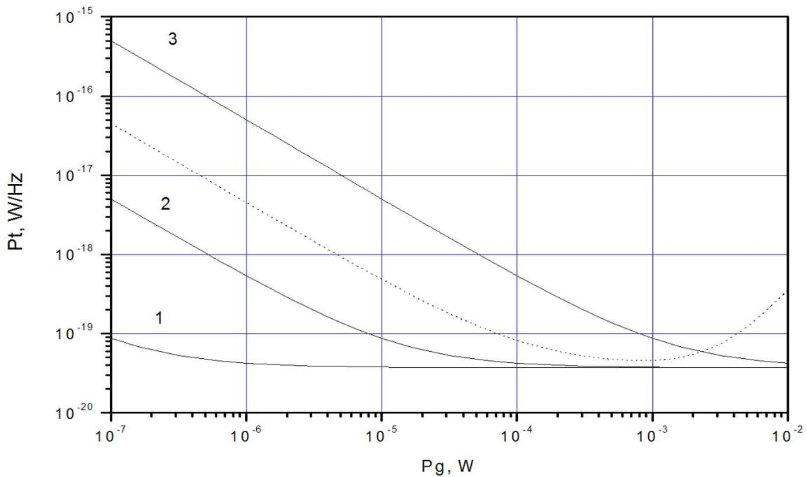
**Figure 37.** The dependences of  $P_t$  on  $P_g$  of HF PD for detection 10,6  $\mu\text{m}$  wavelength radiation at  $\eta = 0,5$ : 1 -  $P_d = 10^{-13}$   $\text{W}/\text{Hz}^{1/2}$ ; 2 -  $P_d = 10^{-12}$   $\text{W}/\text{Hz}^{1/2}$ ; 3 -  $P_d = 10^{-11}$   $\text{W}/\text{Hz}^{1/2}$ .
