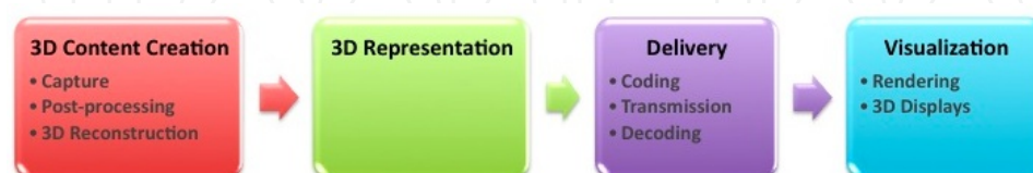
Figure 1. Pipeline of an end-to-end 3D video system.
