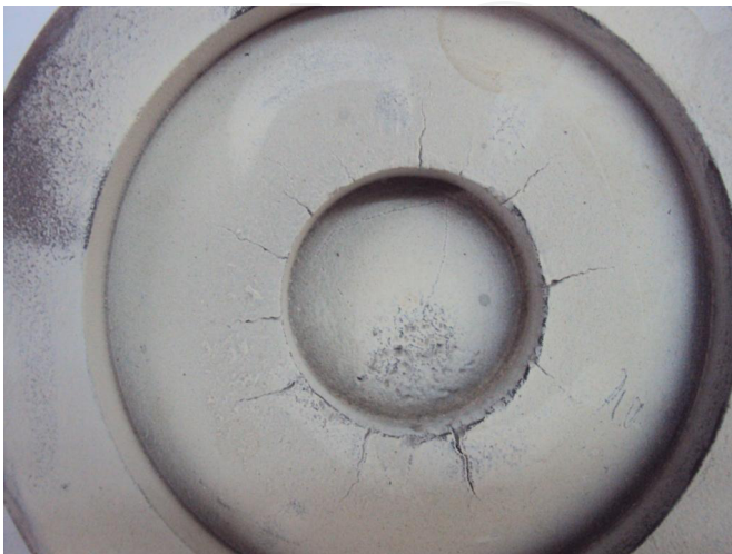
Figure 48. Typical Thermal Fatigue Cracks in a PM.
