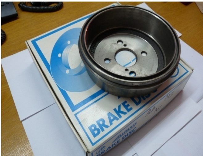
Figure 47. A Brake Drum made by PM process.
