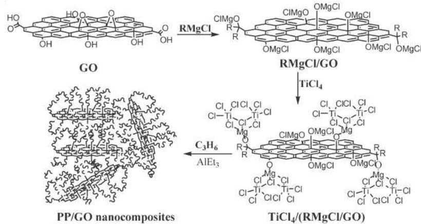
**Figure 6.** Fabrication of PP/GO nanocomposites by in situ Ziegler-Natta polymerization [37].
