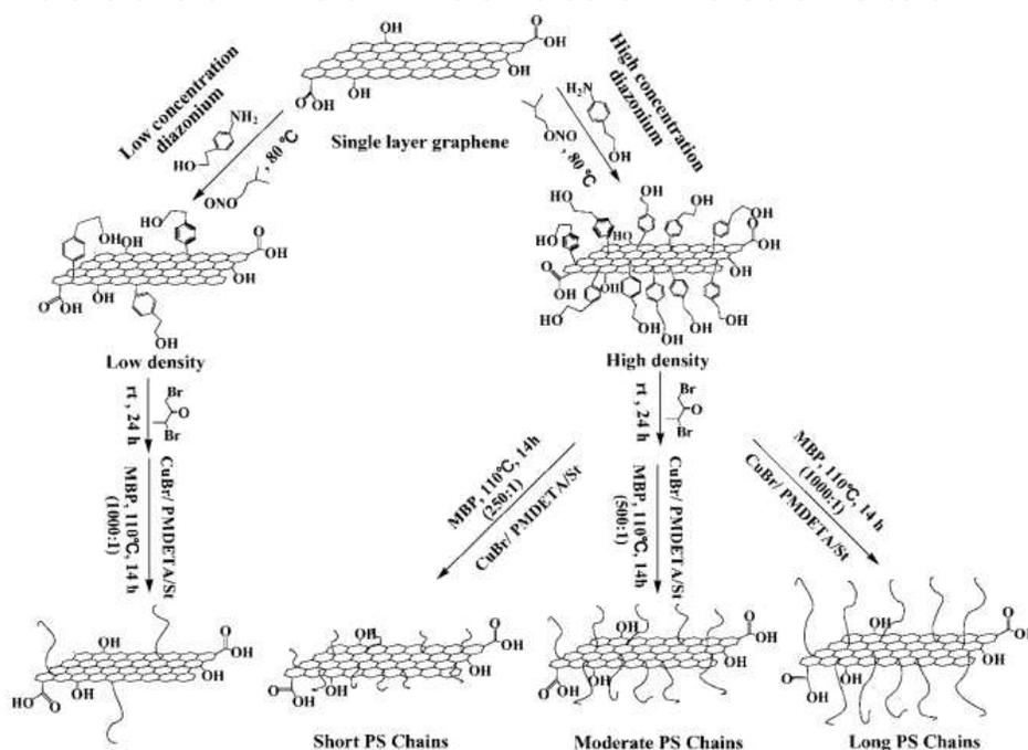
**Figure 2.** Synthetic routes for achieving controllable functionalization of graphene.<sup>28</sup>
