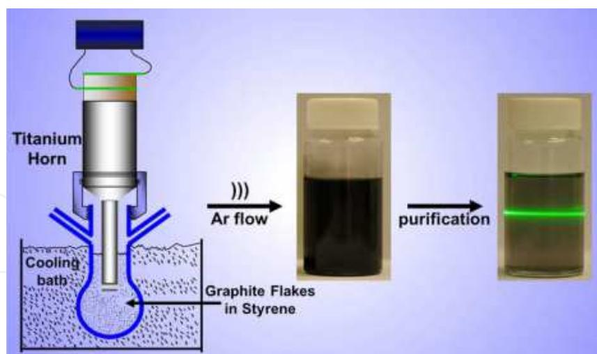
**Figure 7.** Experimental setup of the one-step mechanochemical process for exfoliation of graphite and sonochemical functionalization of graphene [53].
