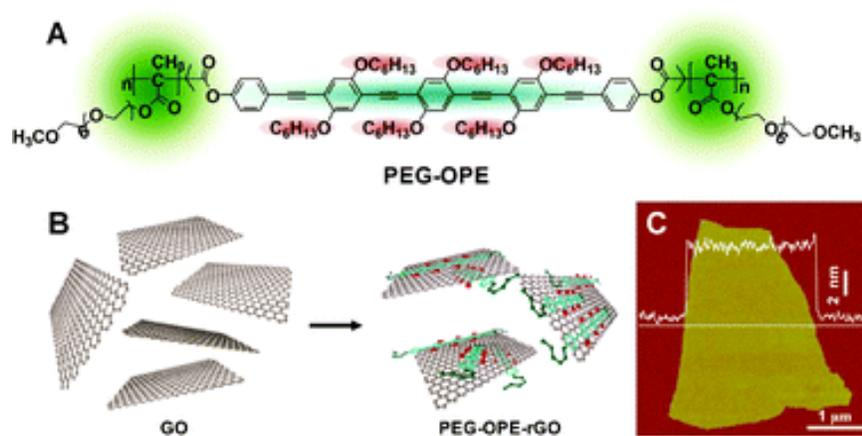
**Figure 18.** A) Chemical structure of PEG-OPE. (B) Schematic illustration of fabrication of PEG-OPE stabilized r-GO sheets. (C) Tapping-mode AFM image and cross-sectional analysis of PEG-OPE-r-GO on mica [67].
