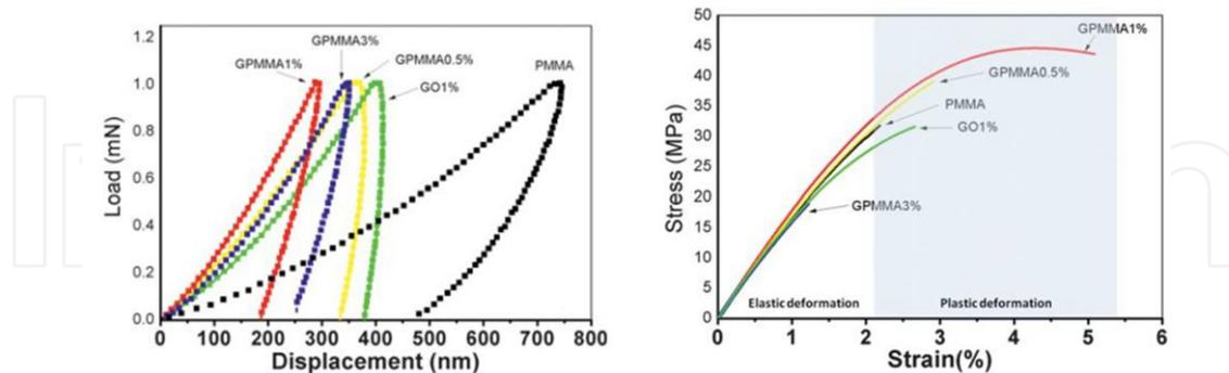
**Figure 3.** Load-displacement nanindentation (left) and stress-strain curves (right) of films of PMMA and its nanocomposites with PMMA-functionalized graphene. <sup>40</sup>
