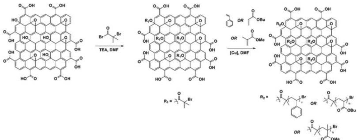
**Figure 1.** Synthesis of surface-functionalized GO via attachment of an ATRP initiator ( $\alpha$ -bromoisobutyryl bromide) followed by polymerization of styrene, butyl acrylate, or methyl methacrylate [38].
