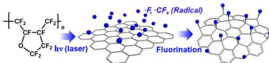
**Figure 10.** The scheme showing a mechanism for fluorination under laser-irradiation.<sup>56</sup>
