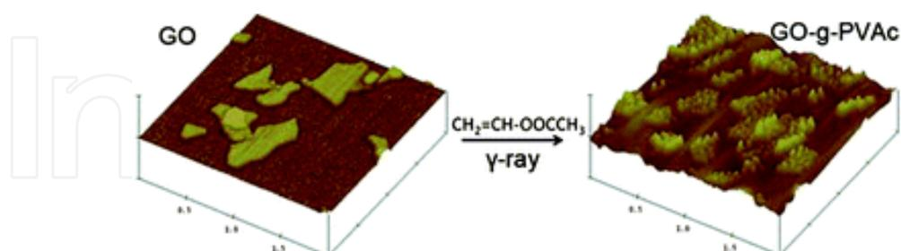
**Figure 9.** The preparation of PVAc grafted GO by  $\gamma$ -ray irradiation-induced graft polymerization [55].
