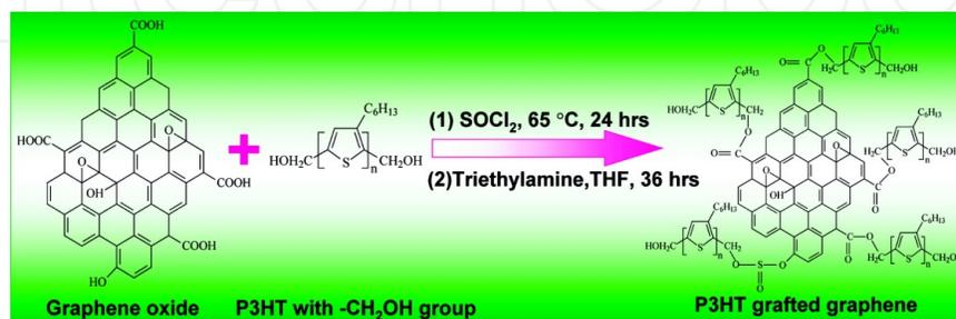
**Figure 13.** Synthesis procedure for chemical grafting of  $\text{CH}_2\text{OH}$ -terminated P3HT chains onto graphene, which involves the  $\text{SOCl}_2$  treatment of GO (step 1) and the esterification reaction between acyl-chloride functionalized GO and  $\text{MeOH}$ -terminated P3HT (step 2) [47].
