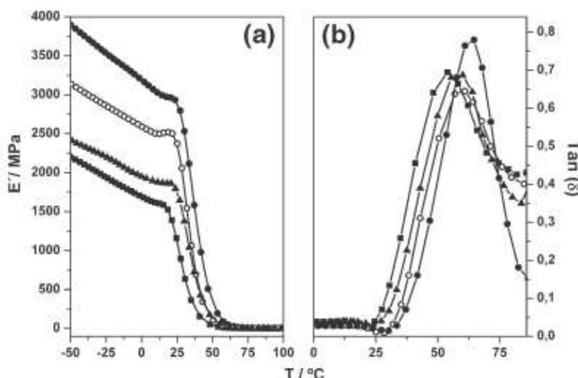
**Figure 12.** Comparison of (a) storage modulus and (b) tan  $\delta$  curves for neat PVC (square), PVC functionalized CNTs (triangle), PVC functionalized GO (solid circle), and PVC functionalized r-GO (open circle) [59].
