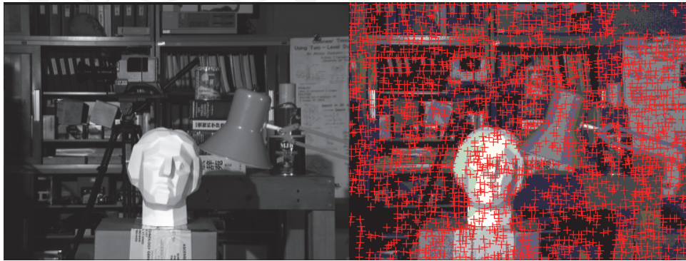
Figure 8. Edge detections in a features-based algorithm.
