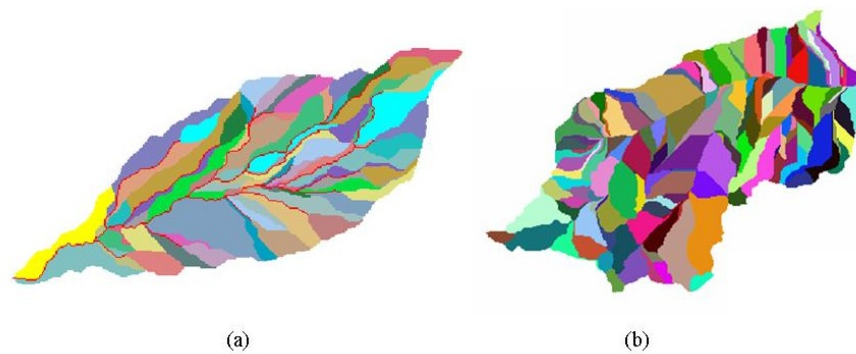
Figure 4. Layouts of the Cannata (left) and Ganspoel (right) watershed discretisation by the AnnAGNPS model.
