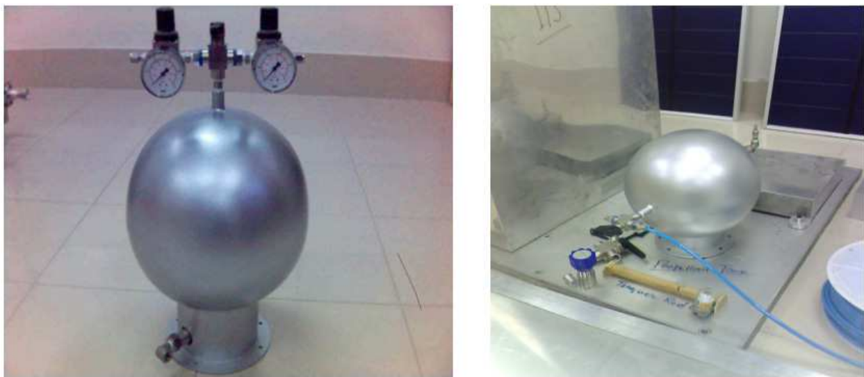
Fig. 8. Installation of Propellant Tank on PRSS Structure
