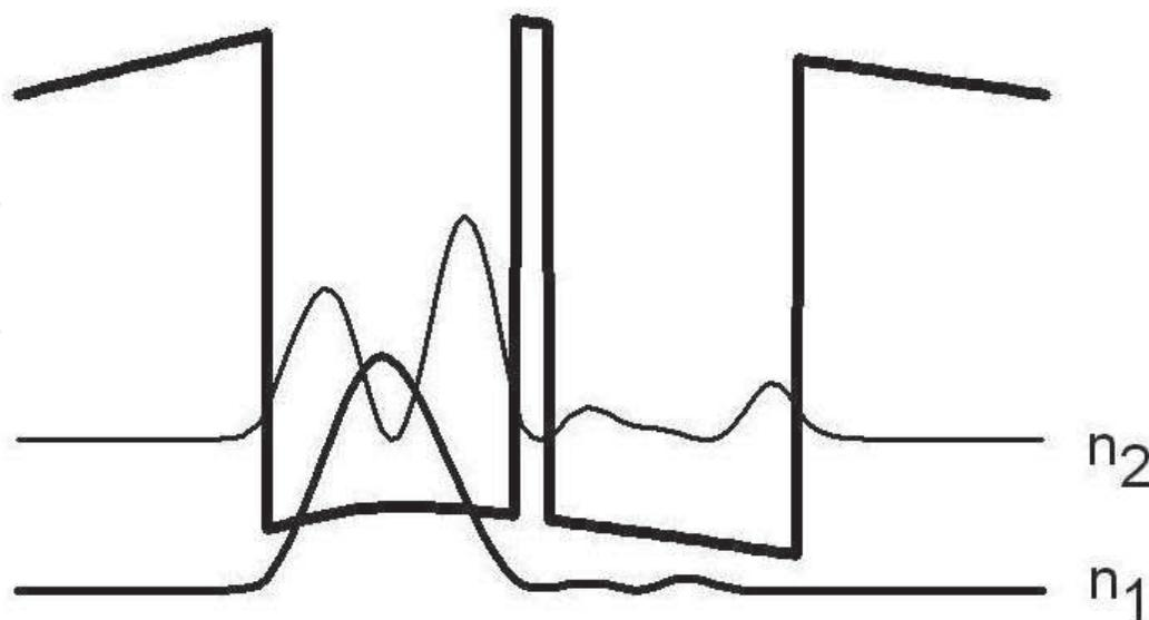
Fig. 2. Conduction band potential and carrier wave functions at  $t = 0.1$  ps. We have taken an initial carrier density equal to  $n_1 = 3.0 \times 10^{11} \text{cm}^{-2}$  and  $n_2 = 0.0 \times 10^{11} \text{cm}^{-2}$ .
