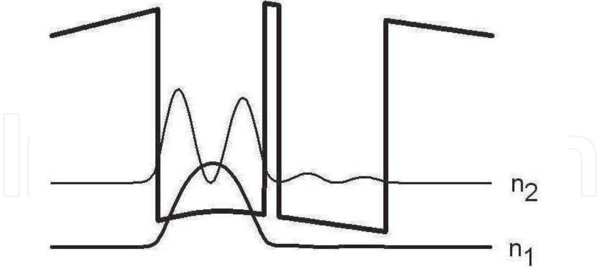
Fig. 3. Conduction band potential and carrier wave functions at  $t = 0.2$  ps. We have taken an initial carrier density equal to  $n_1 = 3.0 \times 10^{11} \text{cm}^{-2}$  and  $n_2 = 0.0 \times 10^{11} \text{cm}^{-2}$ .
