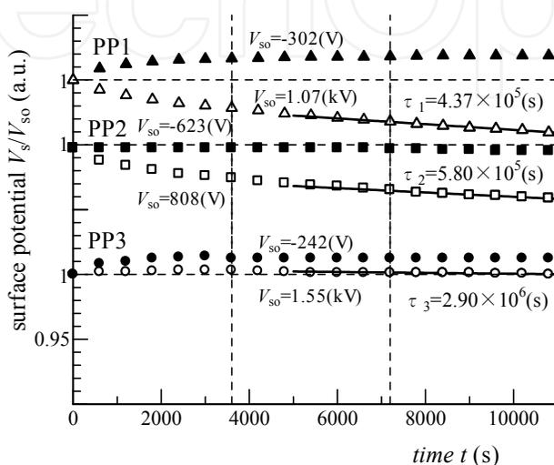
Fig. 16. Isothermal surface potential decay curves for porous and solid PP films at room temperature ( $\blacktriangle, \blacksquare, \bullet$ :negative charged,  $\triangle, \square, \circ$ :positive charged).
