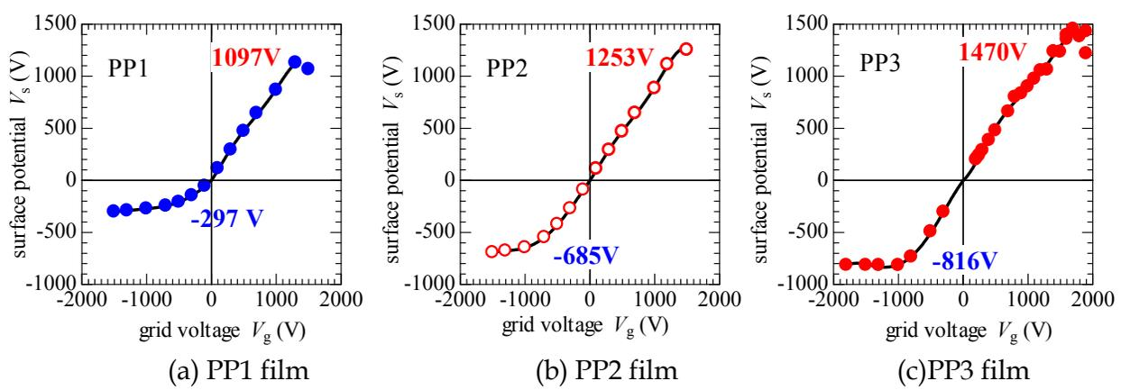
Fig. 14. Grid voltage dependence of the surface potential.
