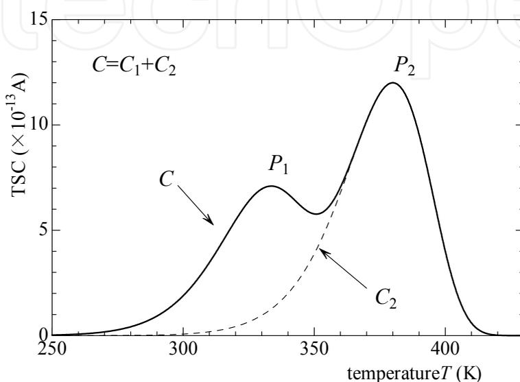
$C_1$  curve:  $E_{t0,1}=0.570$ (eV),  $T_{m0,1}=330.00$ (K),  $I_{m0,1}=6.000(\times 10^{-13}$ A)
