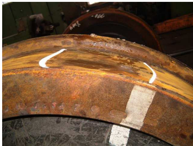
Fig. 1. Flat spot on a wheel tread 1
