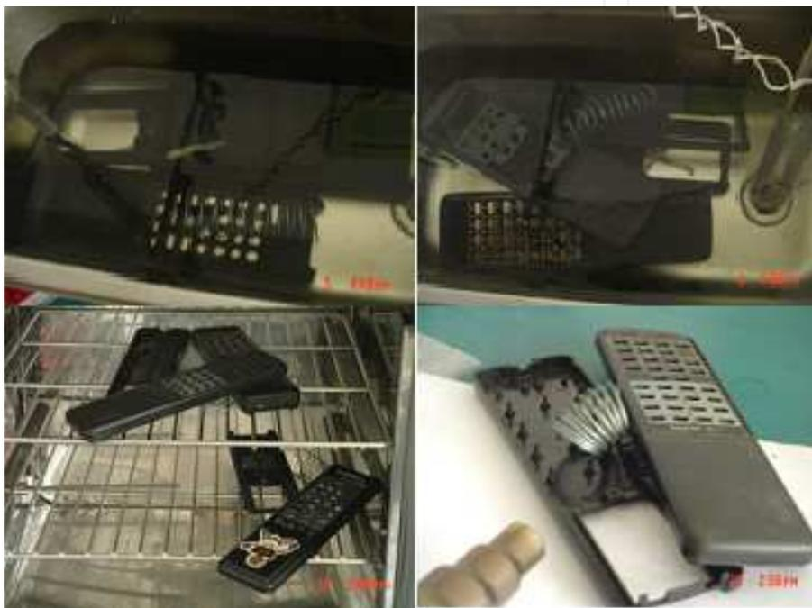
Fig. 1. The active disassembly efficiency of the shells of remote controls (G. Liu et al., 2008).
