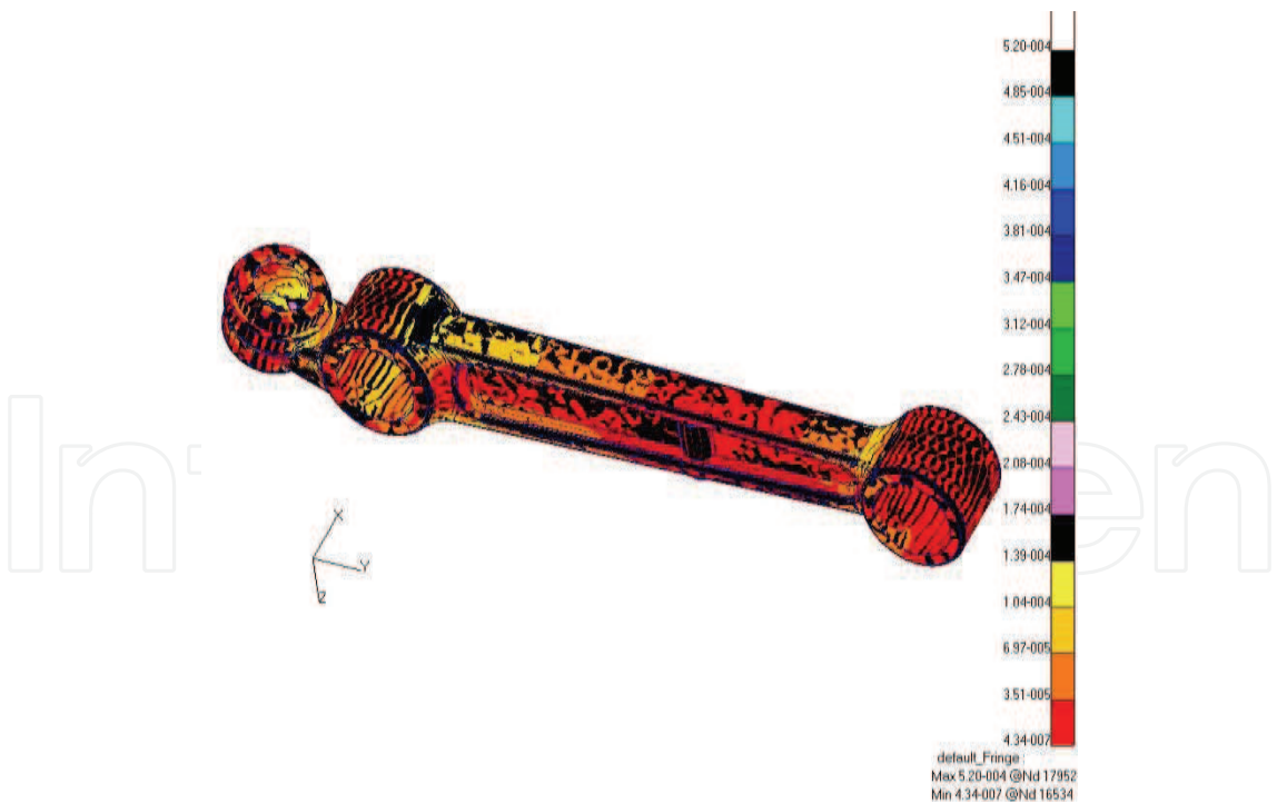
Fig. 5. Stress distribution and strain gauge positions
