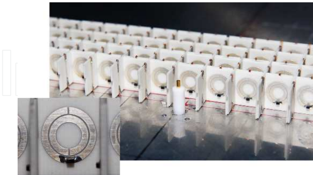
Fig. 14. Photograph of the nonlinear tunable metamaterial created by square arrays of wires and nonlinear SRRs. Each SRR contains a varactor (see the inset) which provides power-dependent nonlinear response.
