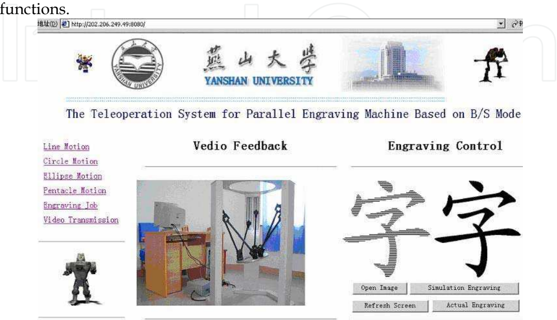
Figure 21. The interface of teleoperation system for engraving
