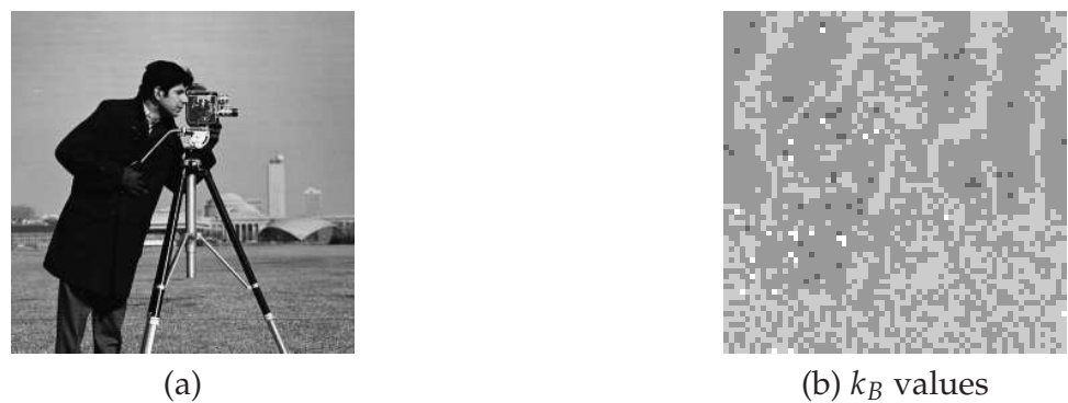
Fig. 16. The embedding parameters k_B that are determined for each block by the adaptive scheme: The block size is 4 \times 4 pels and the threshold S_T = 3.5 ; (a) source image Cameraman of 256 \times 256 8-bit pels; (b) k_B values, black means k_B = 1 and the brighter, the larger k_B .
