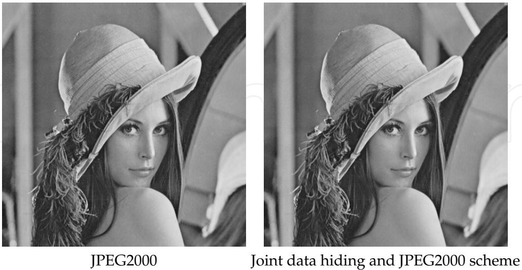
Fig. 8. Comparison between Lena image data hidden and compressed with our joint scheme and the same image compressed with JPEG2000 at 1.6 bpp.
