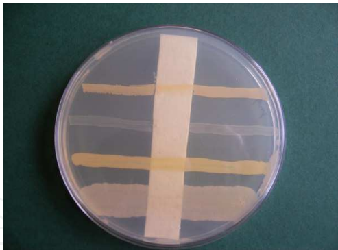
Photo 3. Growth of bacteria respectively from the top: S. aureus , E. coli ; M.flavus , B. licheniformis under polymer with nano-silver - method according to AATCC 147
