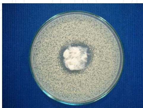
Photo 2. Growth inhibition zone around the C. albicans polypropylene fibers containing 2% Ingaguard- method according to SN 195921
