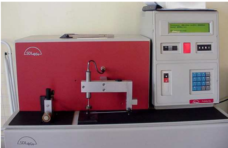
Fig. 5. The step thickness meter SDL M 034/1
