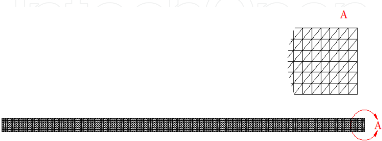
Fig. 4. Mesh for two-dimensional simulations.
