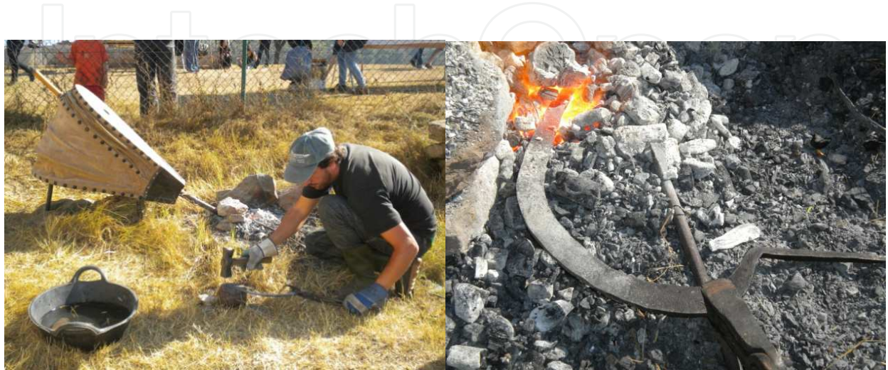
Fig. 16. Experimental process of an iron sickle forging and production
