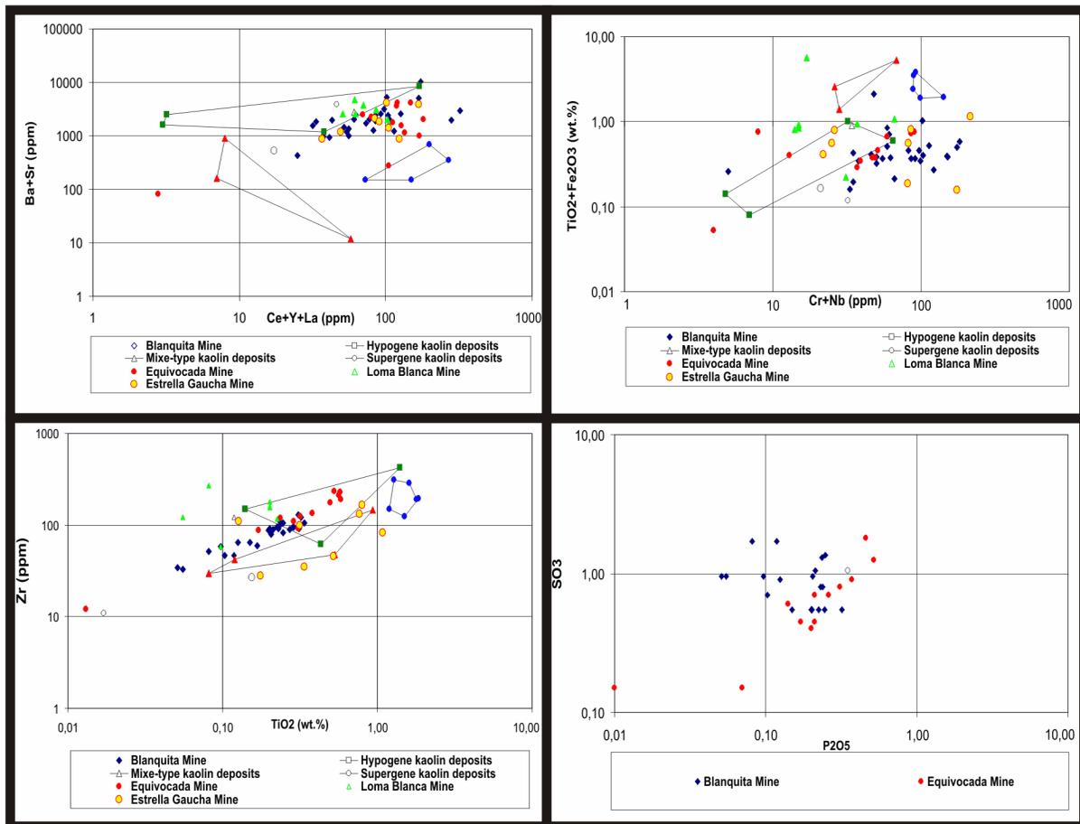
Fig. 5. Data plot from Blanquita, Equivocada, Loma Blanca and Estrella Gaucha mines. a. (Ba + Sr) vs. (Ce + Y + La). b. (TiO<sub>2</sub> + Fe<sub>2</sub>O<sub>3</sub>) vs. (Cr. + Nb) c. Zr vs. TiO<sub>2</sub>. d. SO<sub>3</sub> vs. P<sub>2</sub>O<sub>5</sub> from Blanquita and Equivocada mines.
