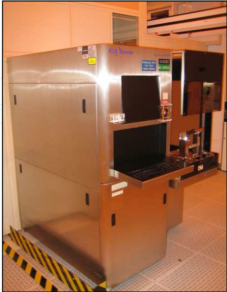
Fig. 11. The SP1 machine which measure the particle
