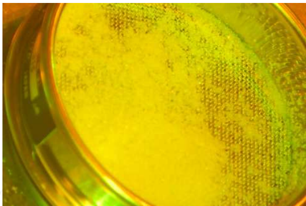
Fig. 6. Appearance of UNH crystal after crystal washing
