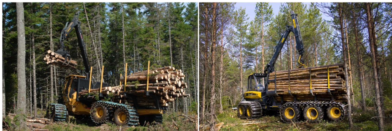
Fig. 8. Eight and ten wheeled forwarder with semi-tracks
