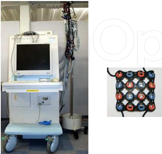
Fig. 4. ETG-7100 system and its shell to hold 4×4 optodes.
