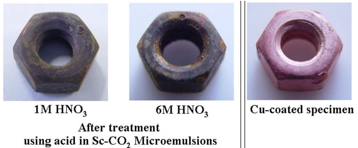
Fig. 16. The photos of specimen before and after acid in Supercritical CO 2 microemulsion treatment.
