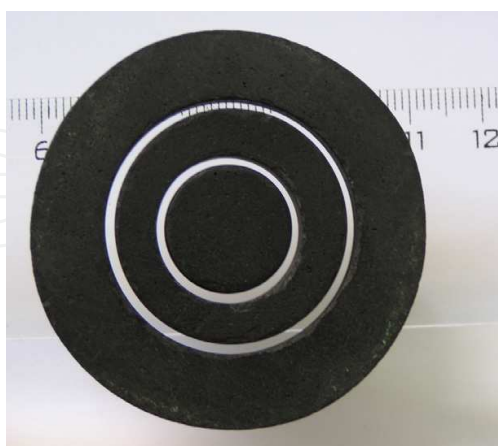
Fig. 1. Rings from YBCO bulk with economical and fast technology
