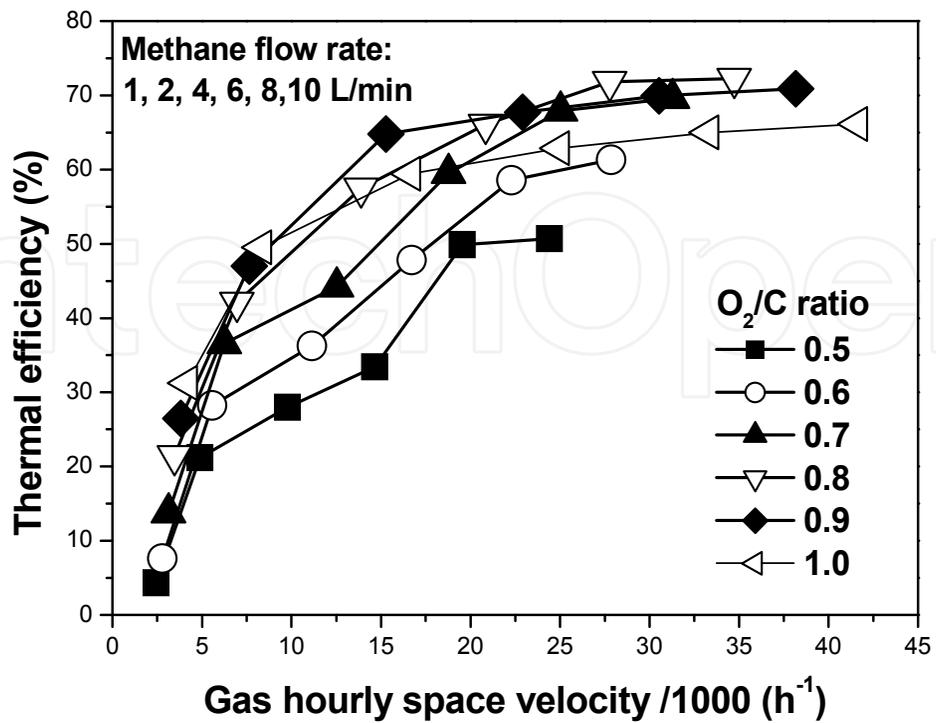
Fig. 12. The effect of space velocity on thermal efficiency at different methane flow rates and O<sub>2</sub>/C ratios
