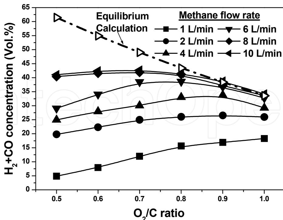
Fig. 7. The influence of O<sub>2</sub>/C ratios on the output concentration of H<sub>2</sub>+CO at different methane flow rates
