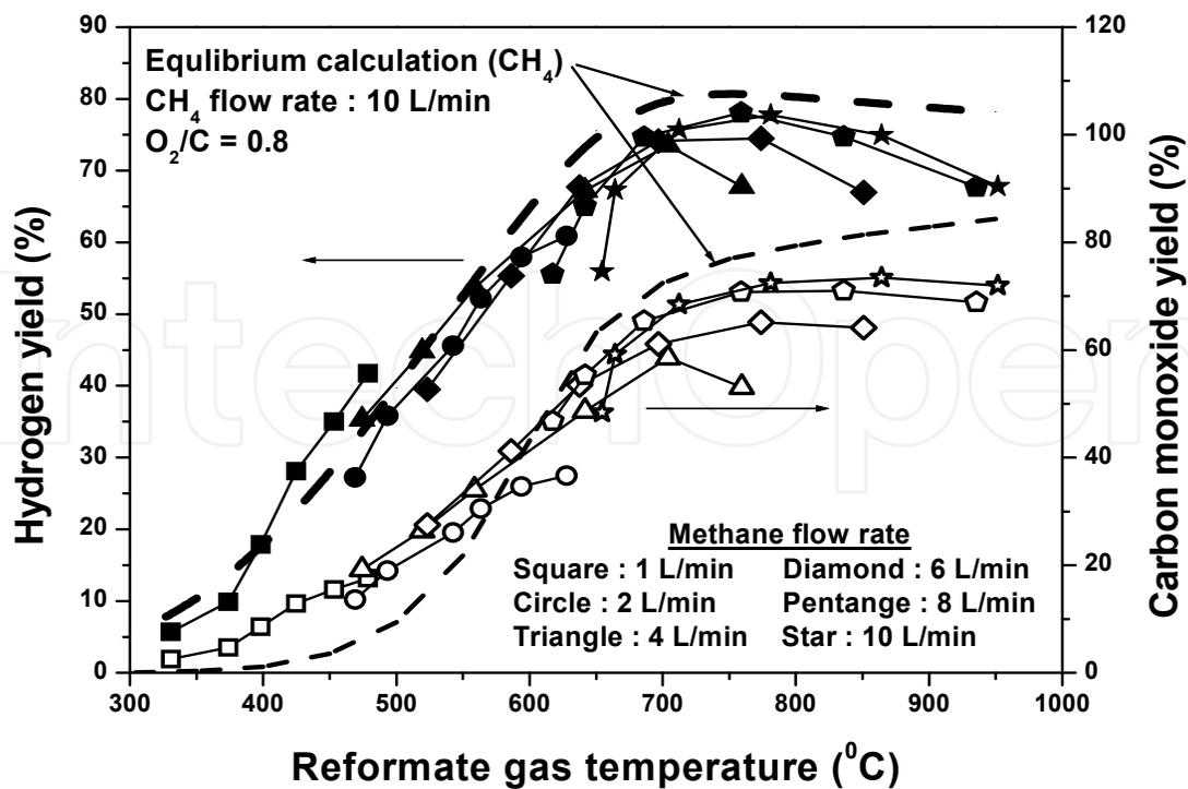
Fig. 11. The relationship between the reformat gas temperature and the yield of H<sub>2</sub> and CO at different methane flow rates
