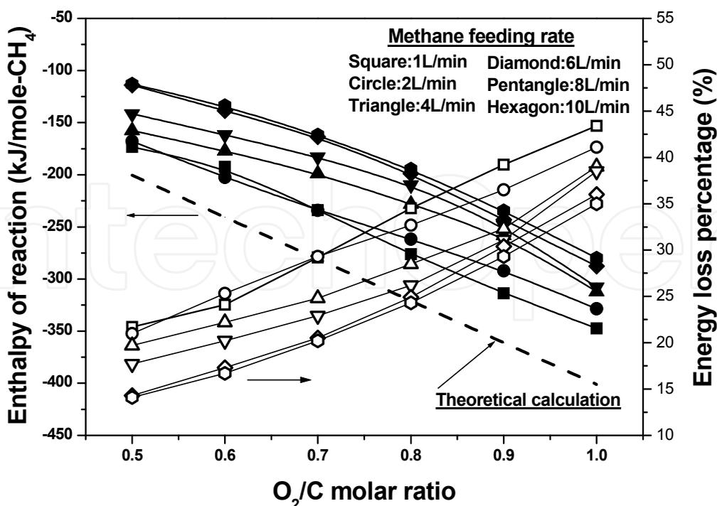
Fig. 8. The relationship between various O<sub>2</sub>/C ratios and the enthalpy of reaction and energy loss percentage at different methane flow rates
