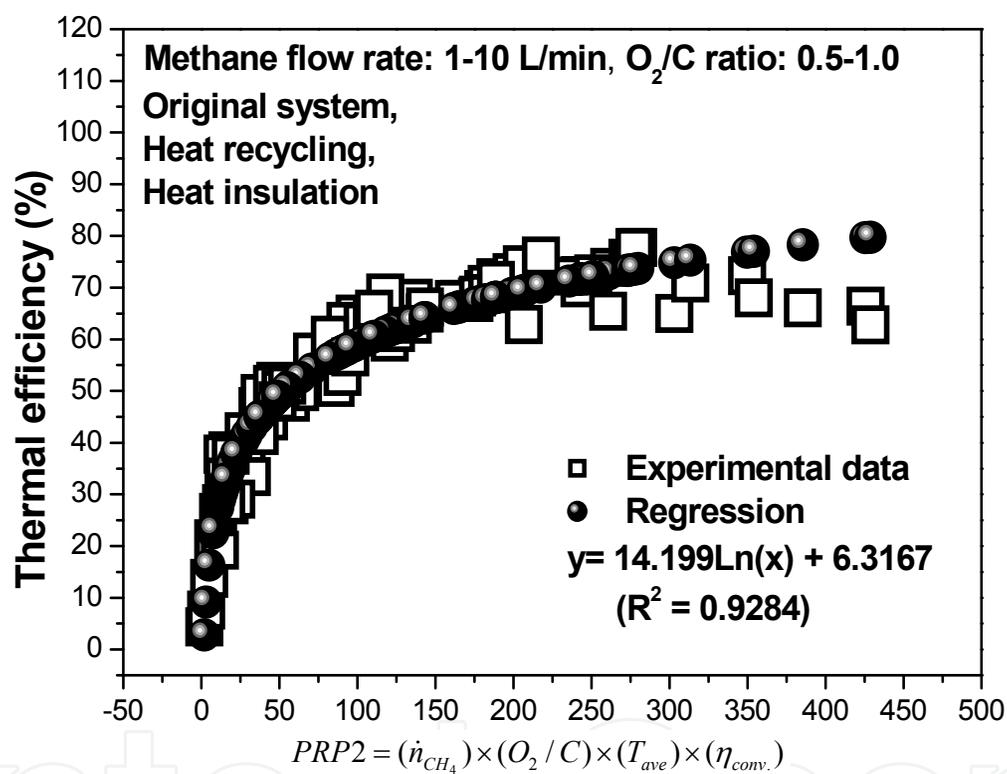
Fig. 17. The effect of the 2<sup>nd</sup> plasma reforming parameters (PRP2) on the total thermal efficiency under different operating conditions
