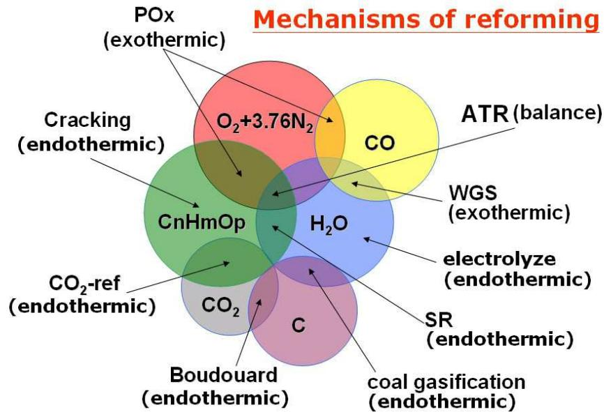
Fig. 4. A relationship chart of reforming mechanisms
