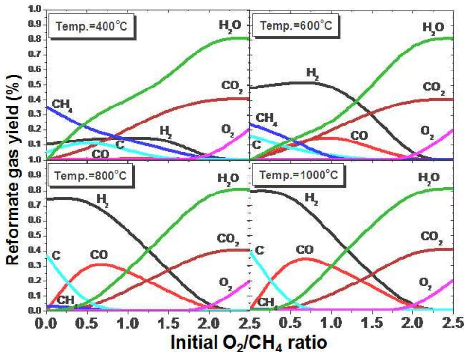
Fig. 5. The variation of the reformat gas yields produced by methane under various O<sub>2</sub>/CH<sub>4</sub> ratios at different reforming temperatures
