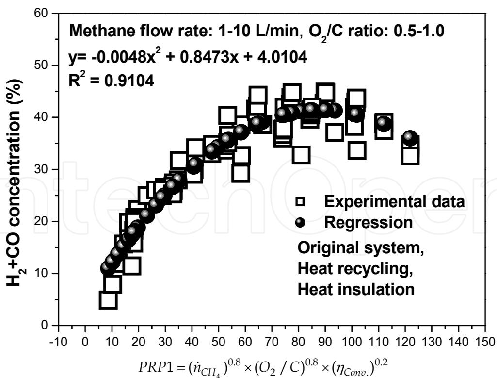
Fig. 16. The effect of the 1<sup>st</sup> plasma reforming parameters (PRP1) on H<sub>2</sub>+CO concentration under different operation conditions
