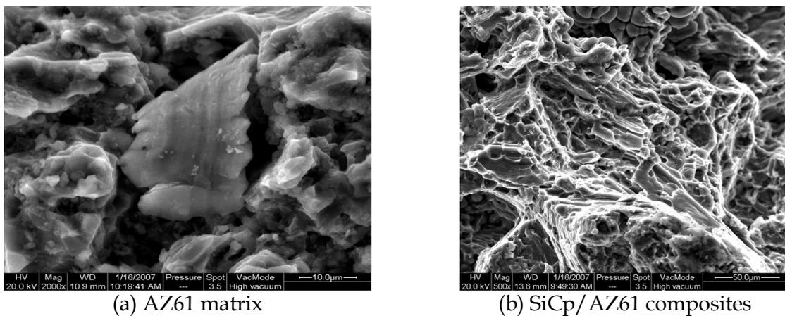
Fig. 6. SEM of tensile fracture surfaces
