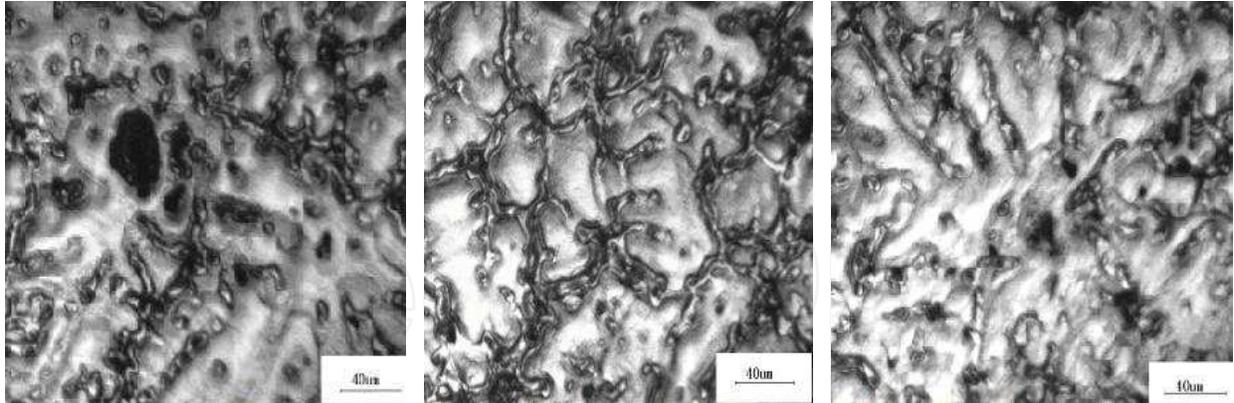
(a) fully-liquid casting process (b) semi-solid casting process (c) stirring-melt casting process
