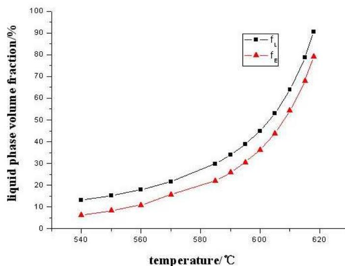
Fig. 8. Relationship between liquid phase volume fraction and temperature
