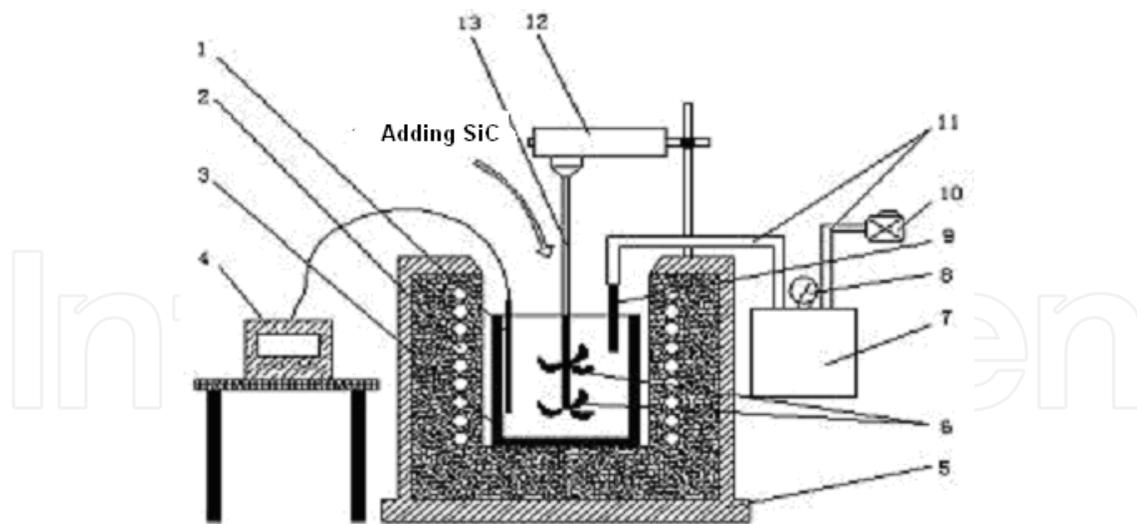
Fig. 1. Schematic diagram of SiCp/AZ61 composites fabricated in stirring casting process 1. thermocouple 2. resistance thread 3. crucible 4. BT608 (artificial aptitude modulator) 5. resistance furnace 6. strapping lamina 7. vacuum jar 8. pressure meter 9. pipette 10. vacuum pump 11. guiding windpipe 12. timing electrical machine 13. stirring bar
