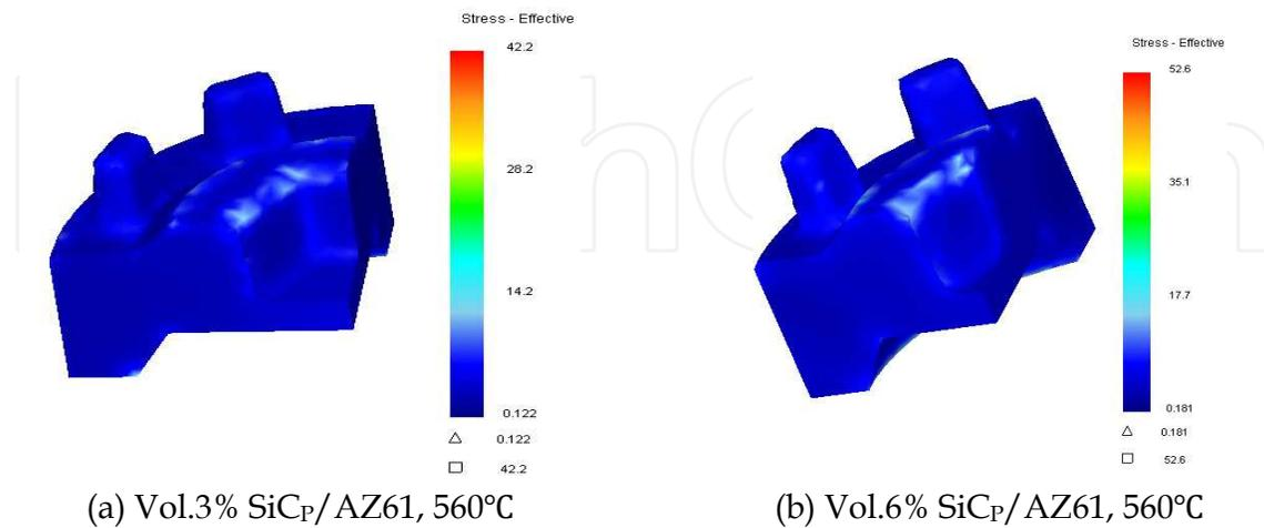
Fig. 24. Effective stress distributions at different volume fraction of SiC particle in thixo-forging process
