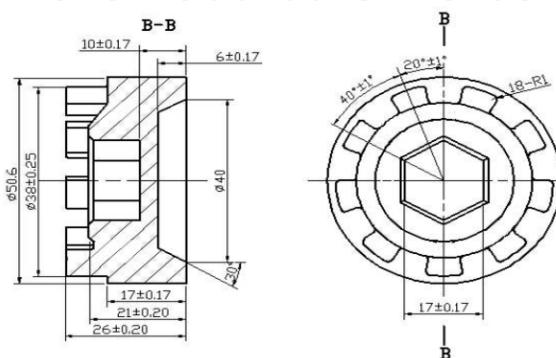
Fig. 20. SiCp/AZ61 composite workpiece
