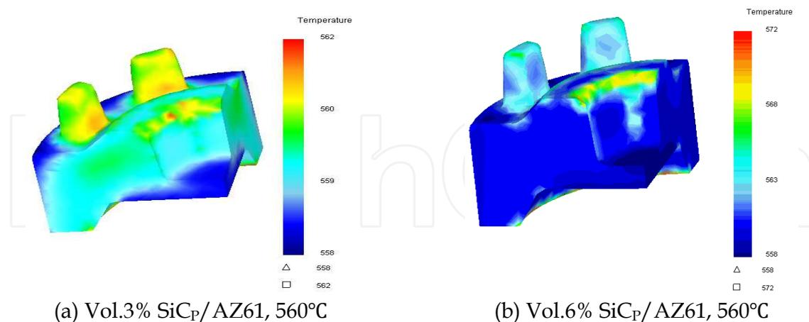
Fig. 25. Temperature distributions at different volume fraction of SiC particle in thixo-forging process
