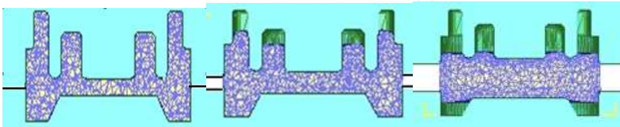
Fig. 21. Filling stages simulated results in thixo-forging process
