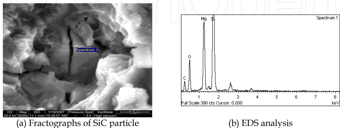
Fig. 7. Fractographs of SiC particle and EDS analysis
