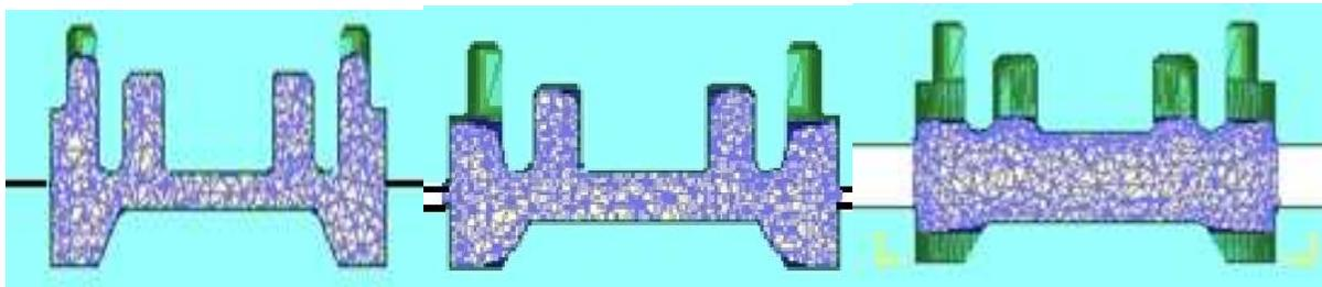
Fig. 22. Filling stages simulated results in forging process
