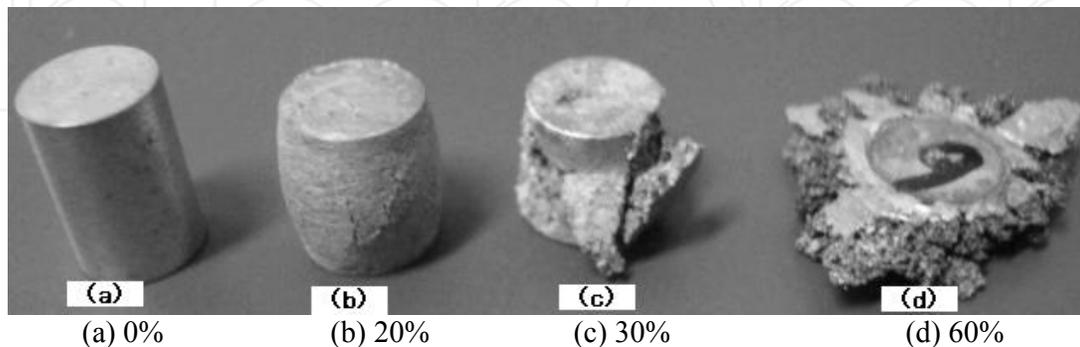
Fig. 17. Appearances of specimens compressed at semi-solid state
