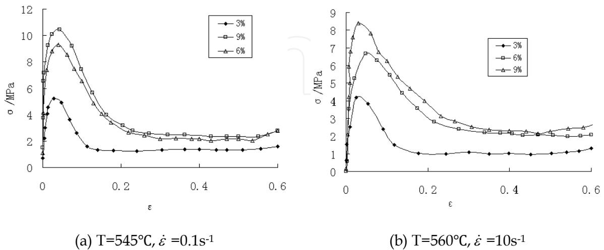
Fig. 16. Curves of stress-strain relation at 545°C and 560°C for SiCp/AZ61 composites with different SiC fractions
