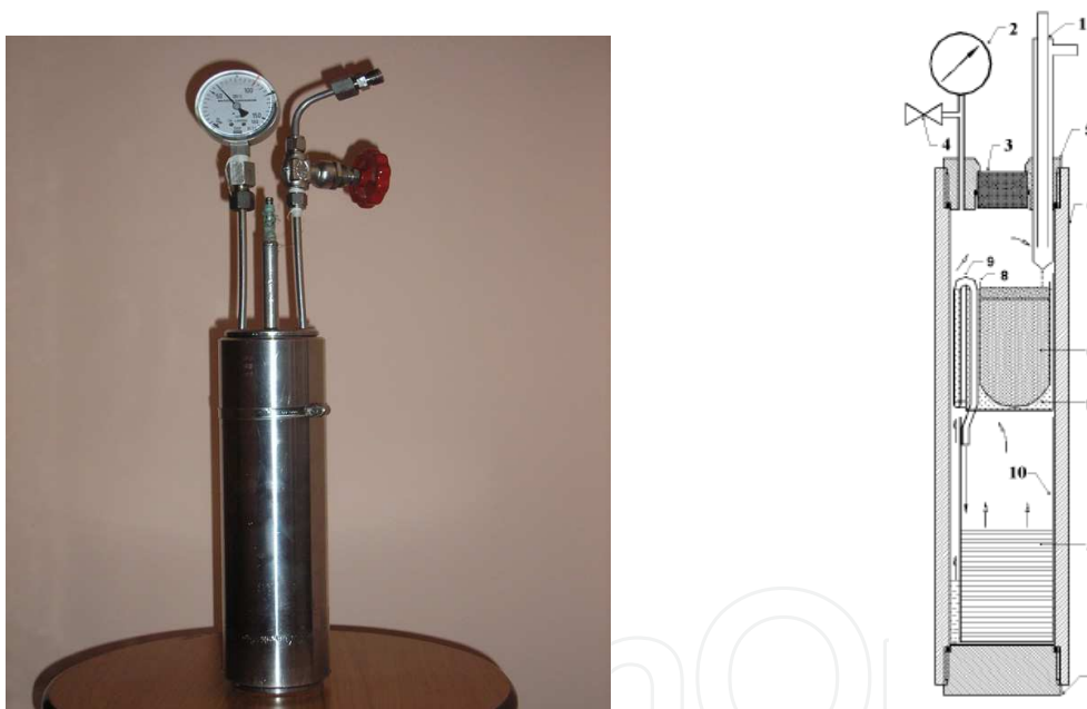
1) Cooling finger; 2) Pressure gauge; 3) Sapphire Window; 4) Valve; 5) Upper cover; 6) Steel Cylinder; 7) Bottom cover; 8) Extracting thimble; 9) Siphon; 10) Product dropping glass; A) Product; B) Extract solution; C) Plant material
