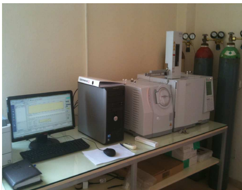
Fig. 5. GC - MS apparatus, used for the chemical composition analyses
