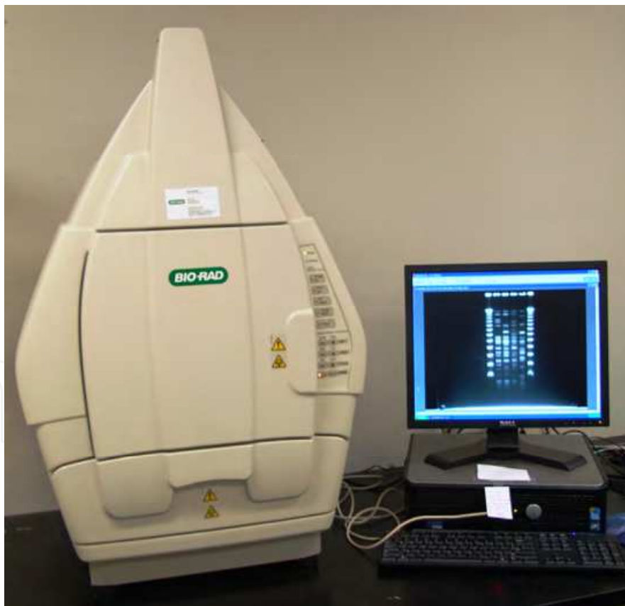
Fig. 2. Picture of Gel Doc (Bio-Rad Hercules, CA, USA) imaging system used to visually analyze images captured after staining the bands formed in the gels.
