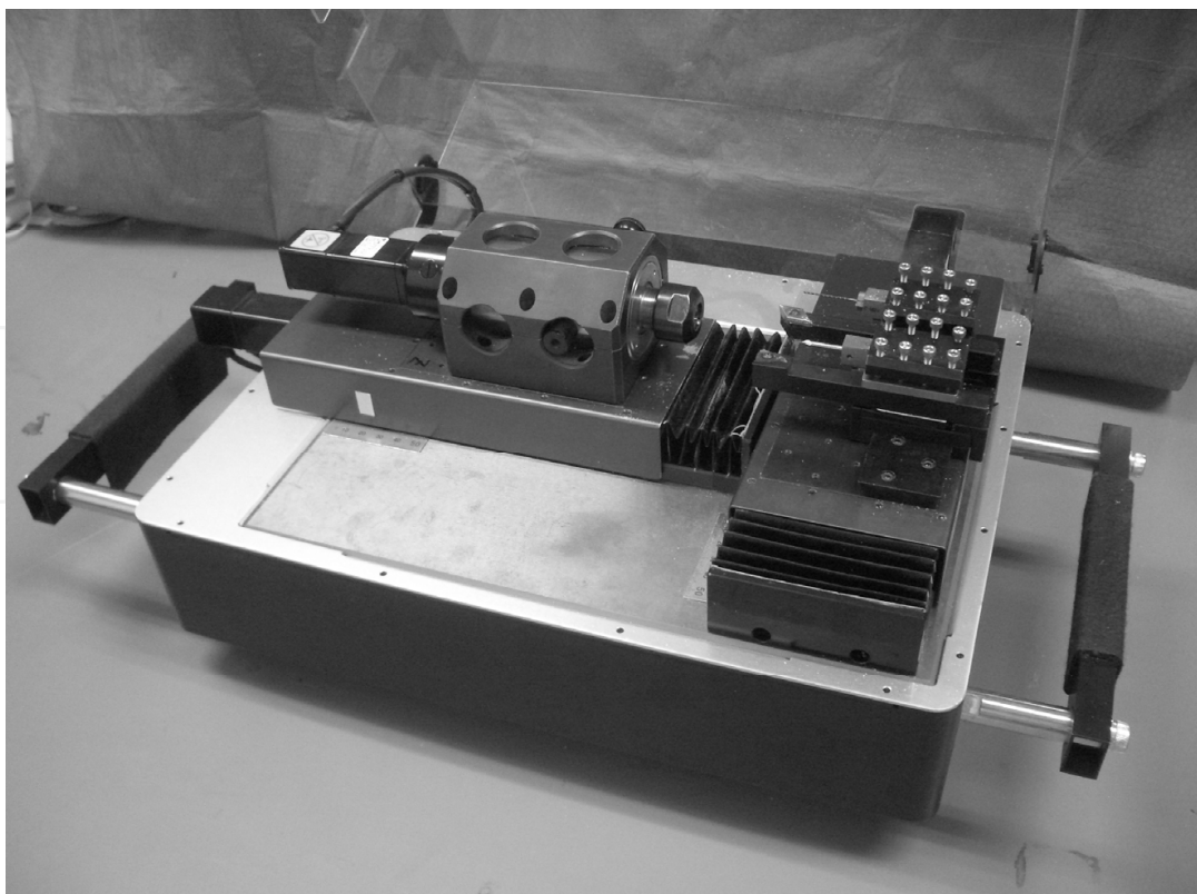
Fig. 1. The precision turning machine developed in this research project.
