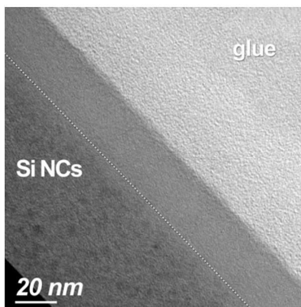
Fig. 16. XTEM micrographs of a two-step annealed  $\text{SiO}_x$  ( $x = 1.3$ ) film with thickness of  $\sim 100$  nm. The contrast observed in the image confirms that the second annealing step (oxidation) forms a free from nanocrystals region with thickness of  $\sim 25$  nm.
