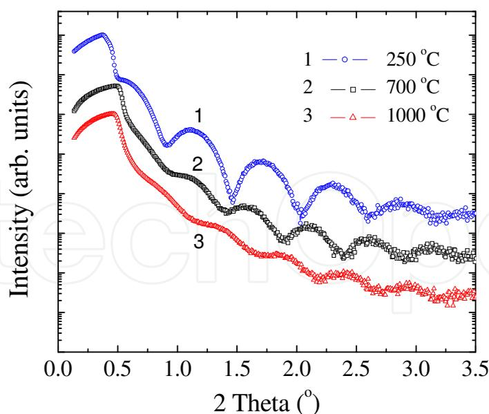
Fig. 5. XRR spectra of a control (1) and annealed at 700 (2) and 1000 °C (3) samples.
