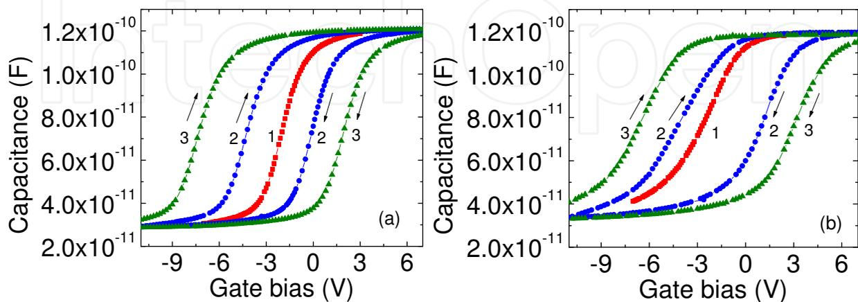
Fig. 9. C-V dependencies measured in the ranges  $\pm 11$  V (curves 2) and  $\pm 15$  V (curves 3) at 1 MHz of samples with (a) amorphous (b) crystalline silicon nanoparticles. The initial curve 1 was measured in the range +3 V, -7 V for both (a) and (b) samples.
