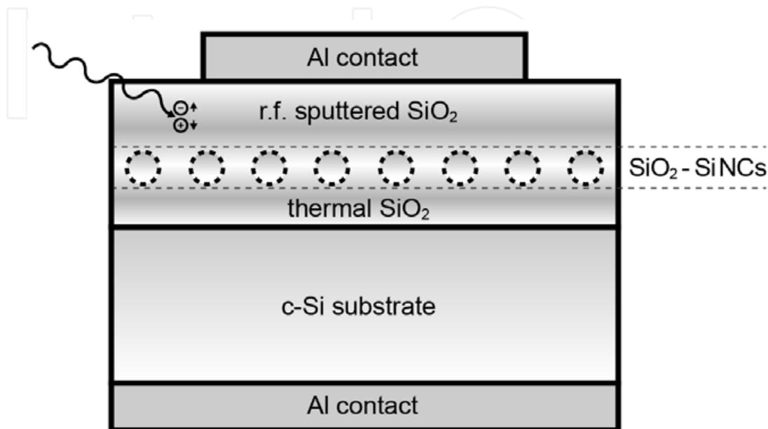
Fig. 12. Schematic cross-section of a MOS structure with three-layer gate dielectric: thermal  $\text{SiO}_2/\text{SiO}_2 - \text{Si NC}/\text{sputtered SiO}_2$ .
